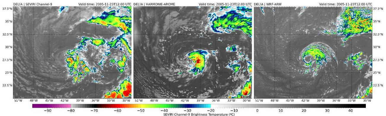
Figure 1: BT (K) spatial distribution for: (left) MSG-SEVIRI satellite, (middle) HARMONIE model, and (right) WRF model for 23 November 2005 at 1200 UTC.
