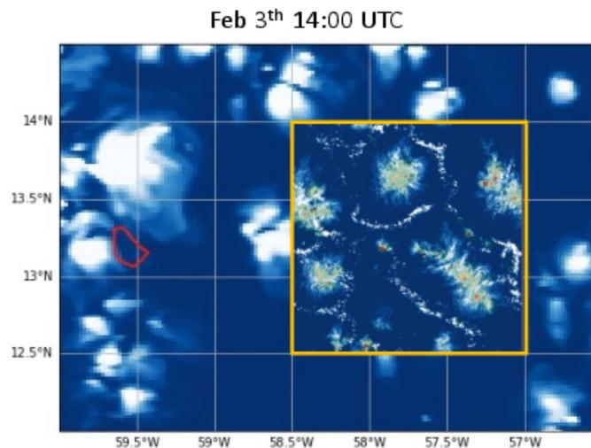
*Figure 1: Snapshot of the simulated liquid water path (LWP) of the mesoscale 2.5km resolution model HARMONIE (outside the orange box) along with the embedded snapshot of LWP simulated by DALES on a 100 meter resolution (inside the box). The red contours indicate the island of Barbados with a typical scale of around 50 km.*
