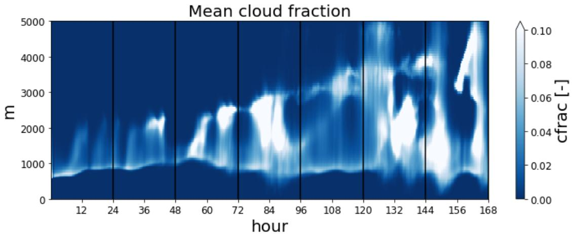
Figure 3: Time development of the cloud fraction of the DALES run without nudging. Note the unrealistic growth of the vertical extent of the cumulus convection
