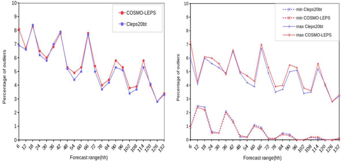
Figure 8: Left panel: Percentage of outliers for different forecast ranges in COSMO-LEPS (red line) and Cleps20bt (blue line). Right panel: Percentage of outliers above/below maximum/minimum predicted values.
