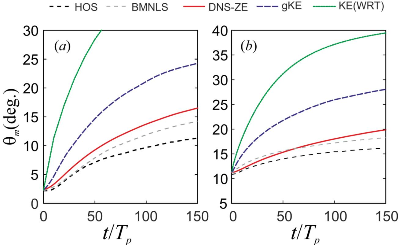
**Figure 2.** Evolution of directional spread  $\theta_m$  (second moment of directional distribution) of two initial spectra (a) A and (b) B. As in figure 1, a direct comparison of five different numerical approaches is shown
