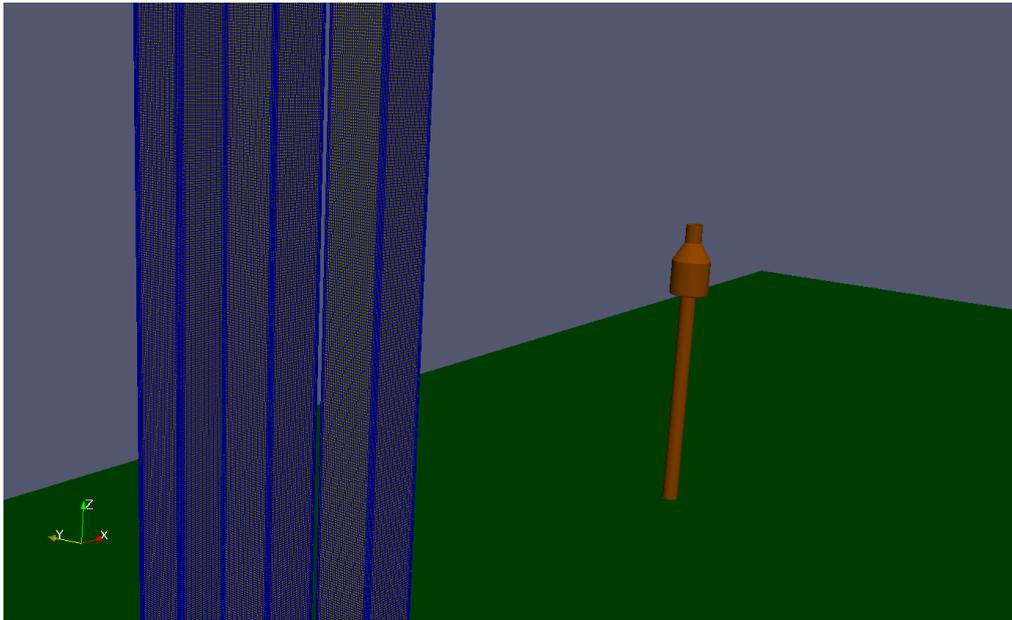
Fig. 4: 3D view of the gauge model and the upwind column used to generate turbulence.
