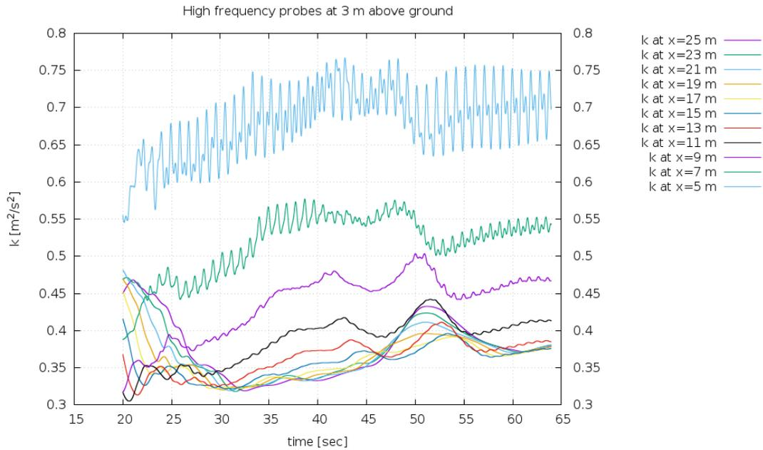
Fig. 6: Time series of the turbulent kinetic energy  $k$  at difference stream-wise distance from the three columns  $U_w = 6$  m/s (URANS simulations).
