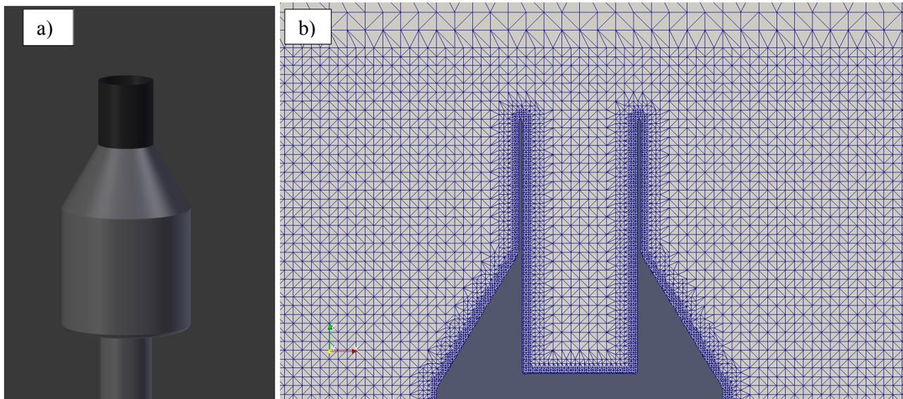
Fig. 3: 3D model of a common unshielded precipitation gauge geometry (panel a). Spatial discretization grid based on polyhedral cells (panel b) on a vertical plane passing through the gauge center.
