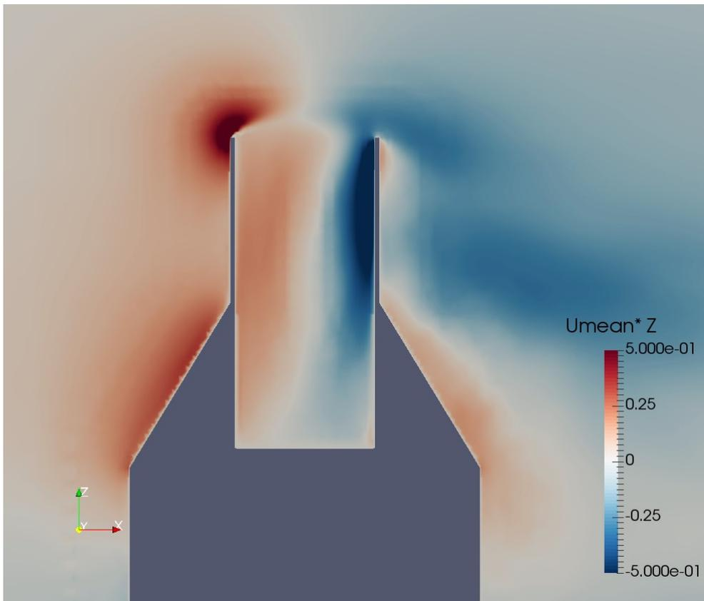
Fig. 8: Mean vertical component of the air velocity near the gauge collector with airflow turbulence (LES simulation results).
