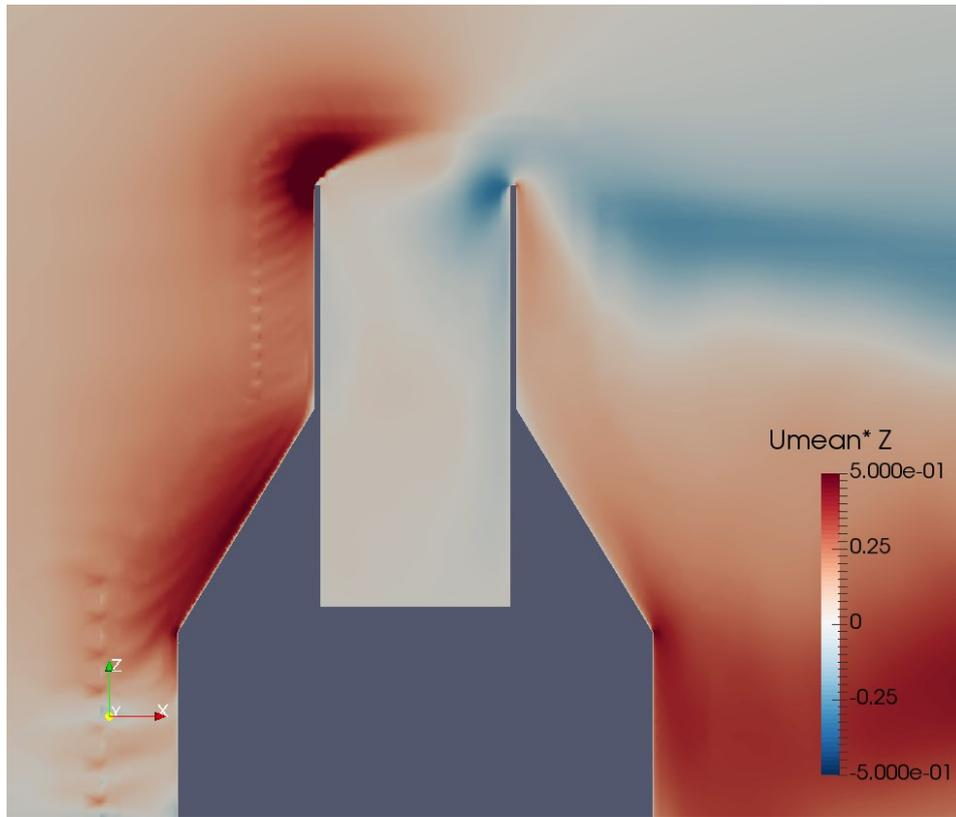
Fig. 7: Mean vertical component of the air velocity near the gauge collector in absence of the airflow turbulence (LES simulation results).
