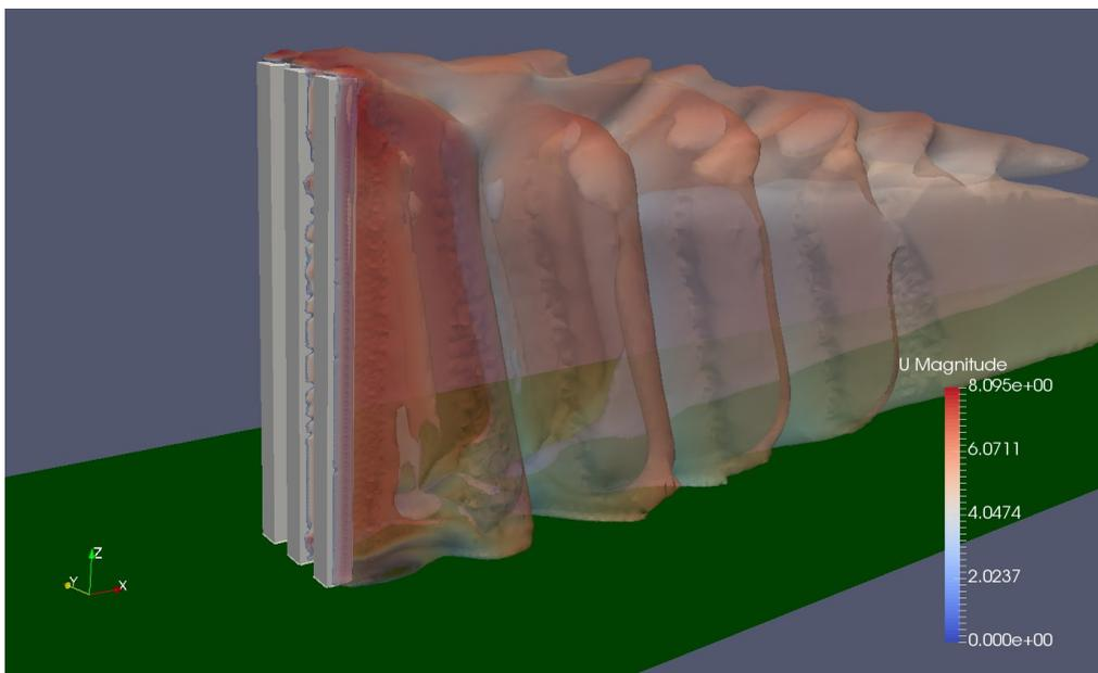
Fig. 5: Contours of the turbulence kinetic energy  $k=0.6 \text{ m}^2/\text{s}^2$  field generated by the three columns under a free stream wind speed  $U_w$  equal to 6 m/s (URANS simulation results).
