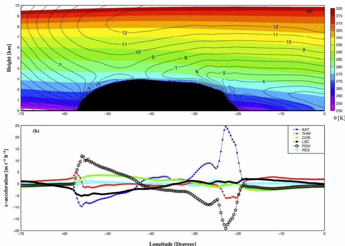
**Figure 1:** Averages for the winter months (1958-2007) for a transect through North Greenland; a: potential temperature and wind speed, b: momentum budget components in the lowest model layer (~7 m).
