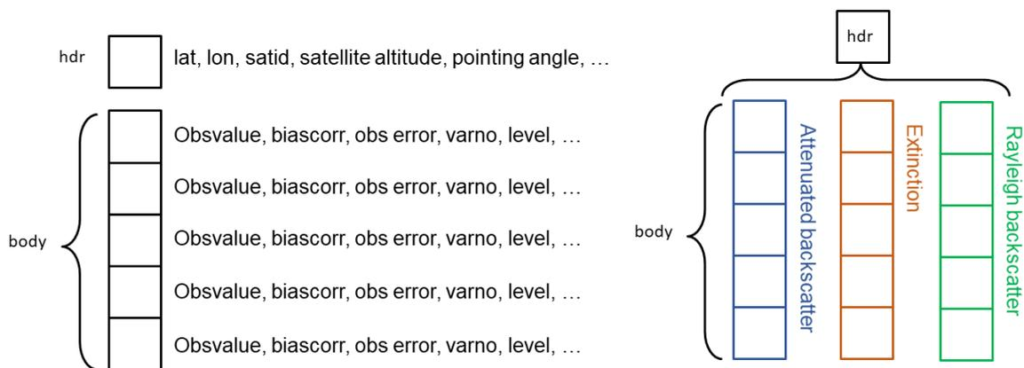
Figure 2.3: Schematic of hdr and body storage within the ODB.
