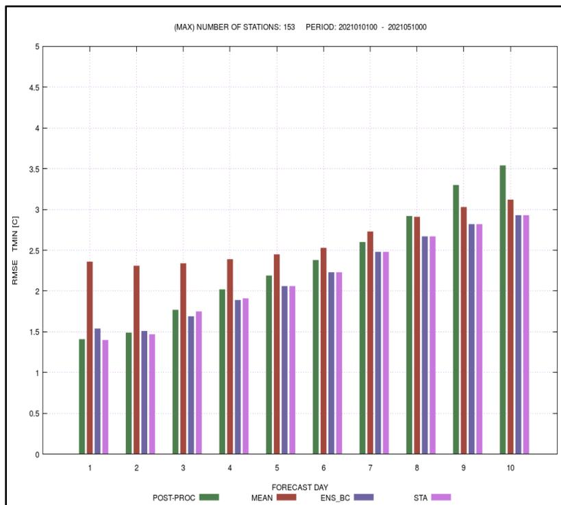
Figure 14: Accuracy of the various components in Portugal’s post-processing and blending system. POST-PROC comes from post-processing HRES, MEAN is the ensemble mean value, ENS\_BC is the ensemble mean post-processed, STA is the final output.
