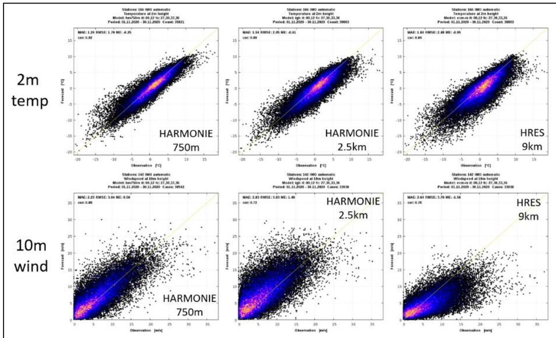
Figure 9: Deterministic run verification scatterplots for Iceland, for 27-36h forecasts, for Nov 2020, for 2m temperature and 10m wind speed (see annotation). Approximately 150 stations were used.
