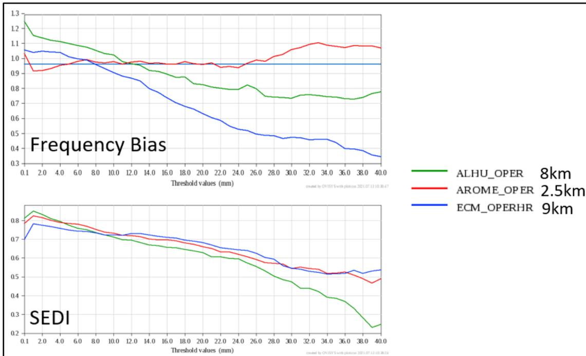
Figure 11: Frequency bias and SEDI (Symmetric Extremal Dependence Index) values of 24h precipitation forecasts (T+6-30h) for 00 UTC runs of HRES (blue), ALADIN (green) and AROME (red) models as a function of precipitation thresholds over Hungary for 2020 using SYNOP observations <400 m above sea level.
