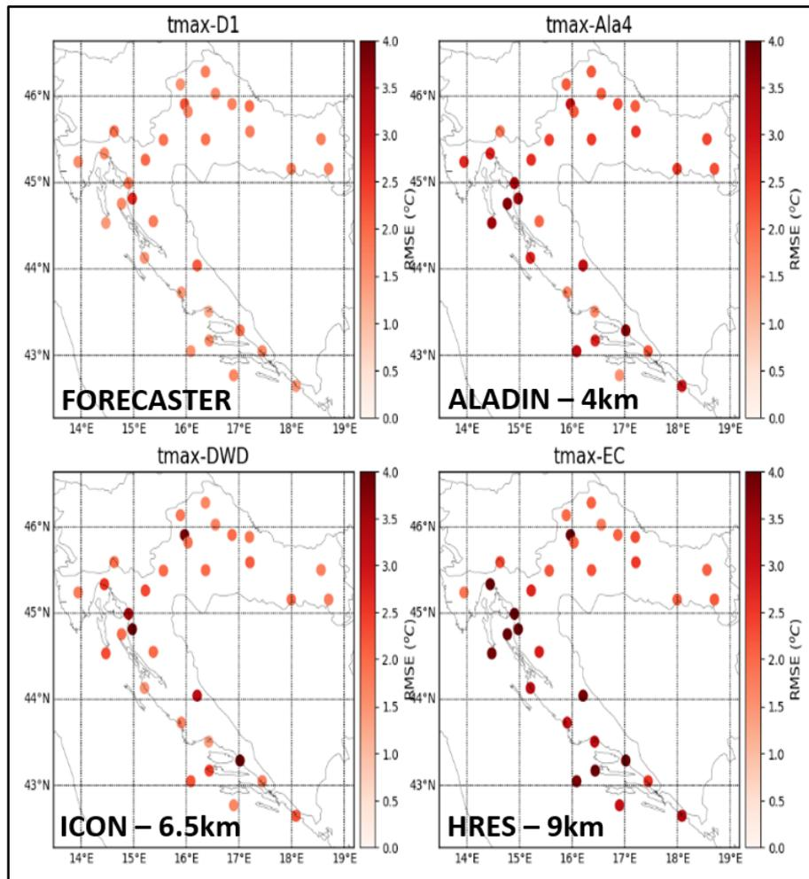
Figure 8: 2m maximum temperature verification (RMSE) for day 2, for Croatia, for 2020, for different models.
