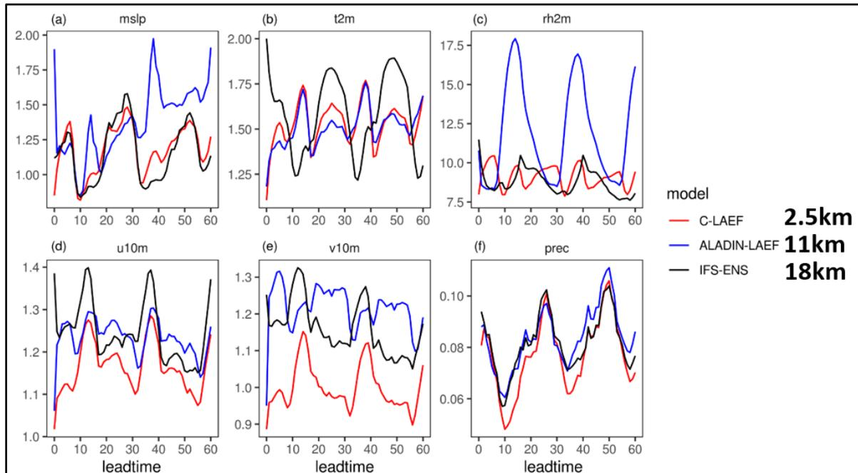
Figure 10: Ensemble verification results (CRPS) for Austria, for Feb/Mar 2020, for 6 parameters (panels (a)...(f) see annotation), versus lead time. Note the clear benefit, for 10m u and v wind components, of 2.5km model resolution.
