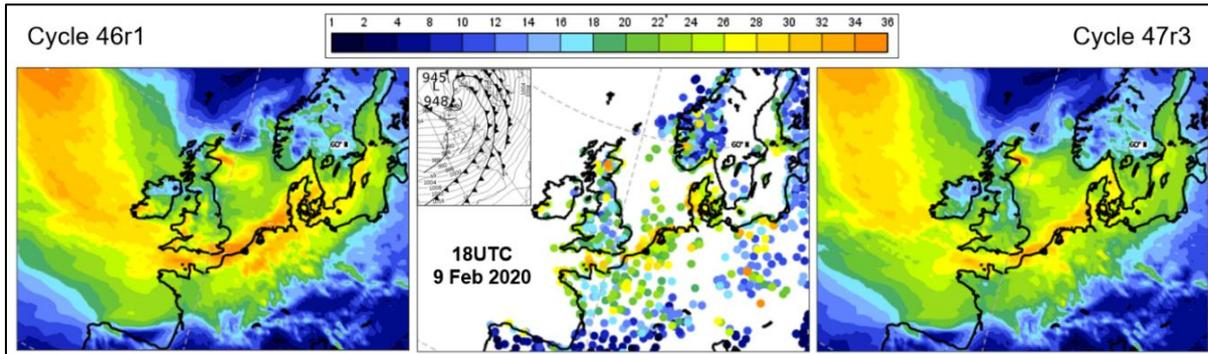
Figure 19: 18h forecasts of gust strength from HRES, valid 18UTC 9 Feb 2020, using cycle 46r1 (left) operational at the time, and cycle 47r3 (right). Observations are also shown, along with a segment of a Met Office synoptic chart for the same time. The scale is in m/s.
