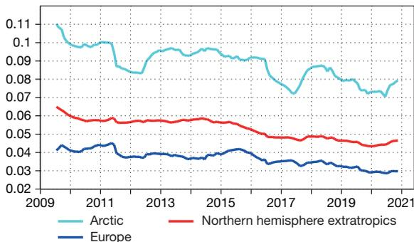
**Figure 1** Fraction of large 2-metre temperature errors in the ECMWF operational ensemble forecasts (with CRPS values larger than 5 K) at day 5 for the Arctic, the northern hemisphere extratropics and Europe.
