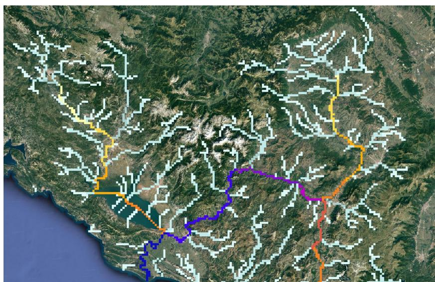
**River drainage network.** The figure shows the LISFLOOD 1 km river drainage network for catchments in northern Albania. Each grid box is coloured according to the upstream drained area, ranging from 25 km<sup>2</sup> (the lightest colour) to more than 14,400 km<sup>2</sup> (dark blue).
