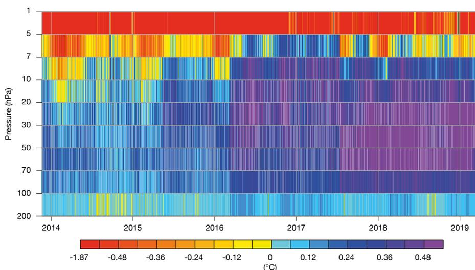
**FIGURE 1** Successive model changes have led to large temperature biases in parts of the stratosphere in the short-range forecasts used in ECMWF's data assimilation system. The chart shows how such biases have evolved since 2014 as measured against temperature retrievals from radio occultation satellite data.
