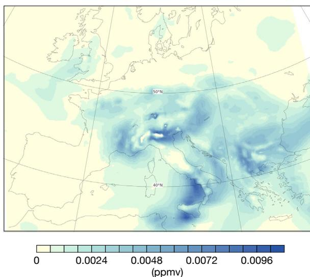
**WRF-Chem example plot.** Initial nitric acid ( $\text{HNO}_3$ ) concentration on the WRF-Chem grid at model level 5, interpolated from CAMS data and plotted in Metview.
