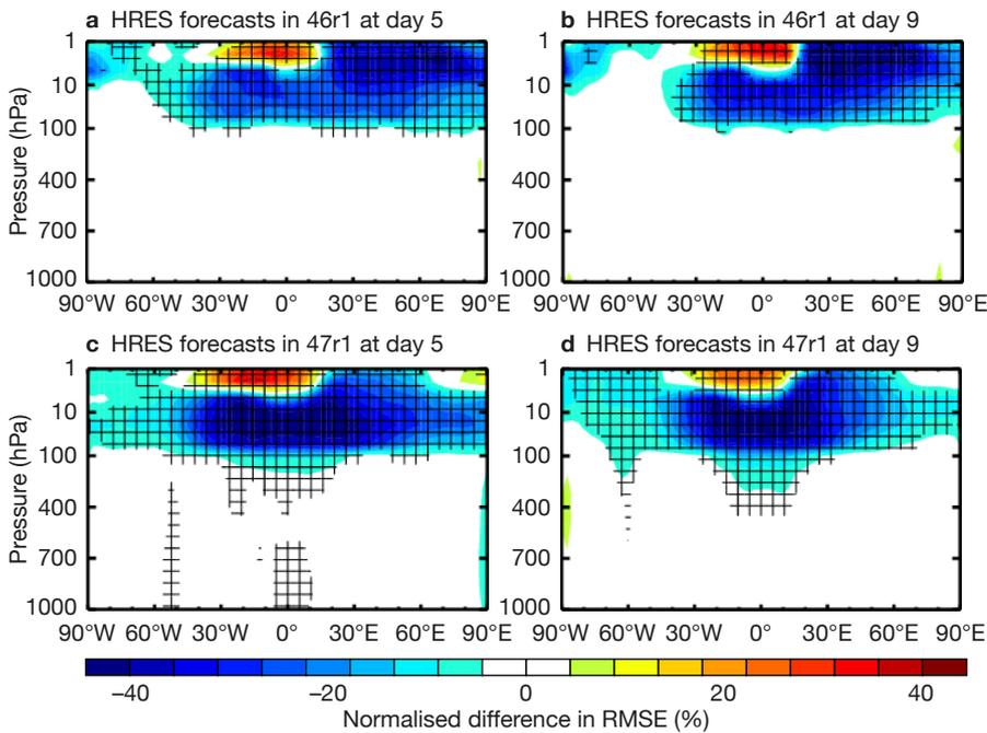
**FIGURE 5** Change in root-mean-square error (RMSE) of geopotential height forecasts when moving from cubic to quintic vertical interpolation. The panels (a) to (d) show the same experiments as detailed for Figure 4. Blue colours indicate that errors are smaller when quintic vertical interpolation is used. Hatched areas indicate statistical significance at an estimated 90% confidence level.
