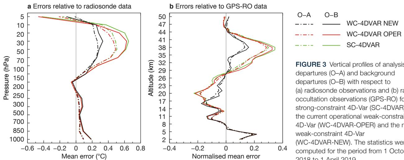
**FIGURE 3** Vertical profiles of analysis departures (O–A) and background departures (O–B) with respect to (a) radiosonde observations and (b) radio occultation observations (GPS-RO) for strong-constraint 4D-Var (SC-4DVAR), the current operational weak-constraint 4D-Var (WC-4DVAR-OPER) and the new weak-constraint 4D-Var (WC-4DVAR-NEW). The statistics were computed for the period from 1 October 2018 to 1 April 2019.
