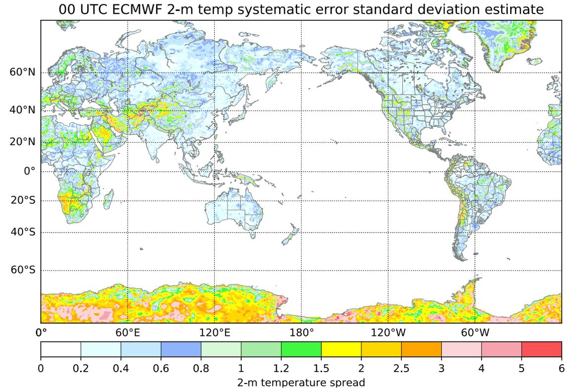
Notable potential systematic errors in ECMWF surface temperature initialization:
