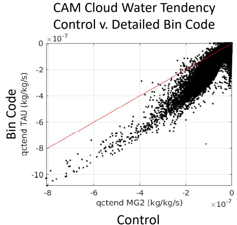
Detailed 'TAU' bin code produces similar changes in cloud water to existing approach, but different structure.
