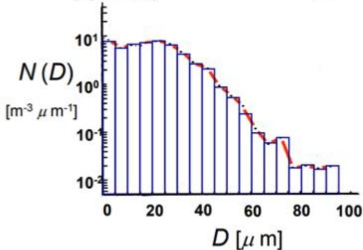
Divide microphysical particles into bins for different sizes, and compute evolution of each bin separately
