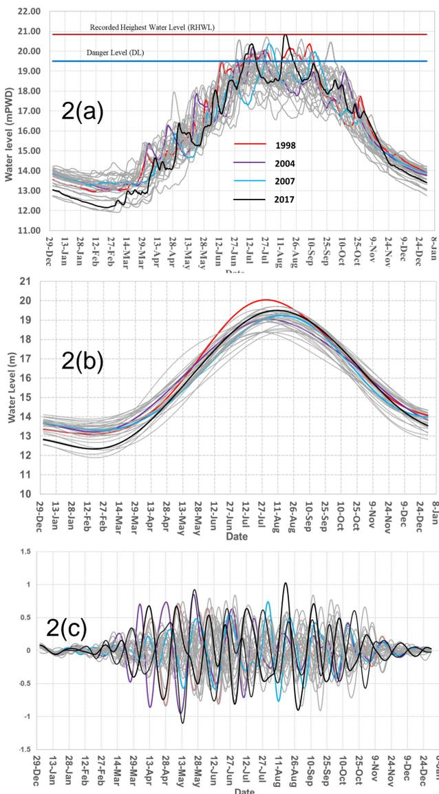
**Figure 2:** a. Full hydrograph (top) b. low frequency component (middle), c. high frequency component (bottom)
