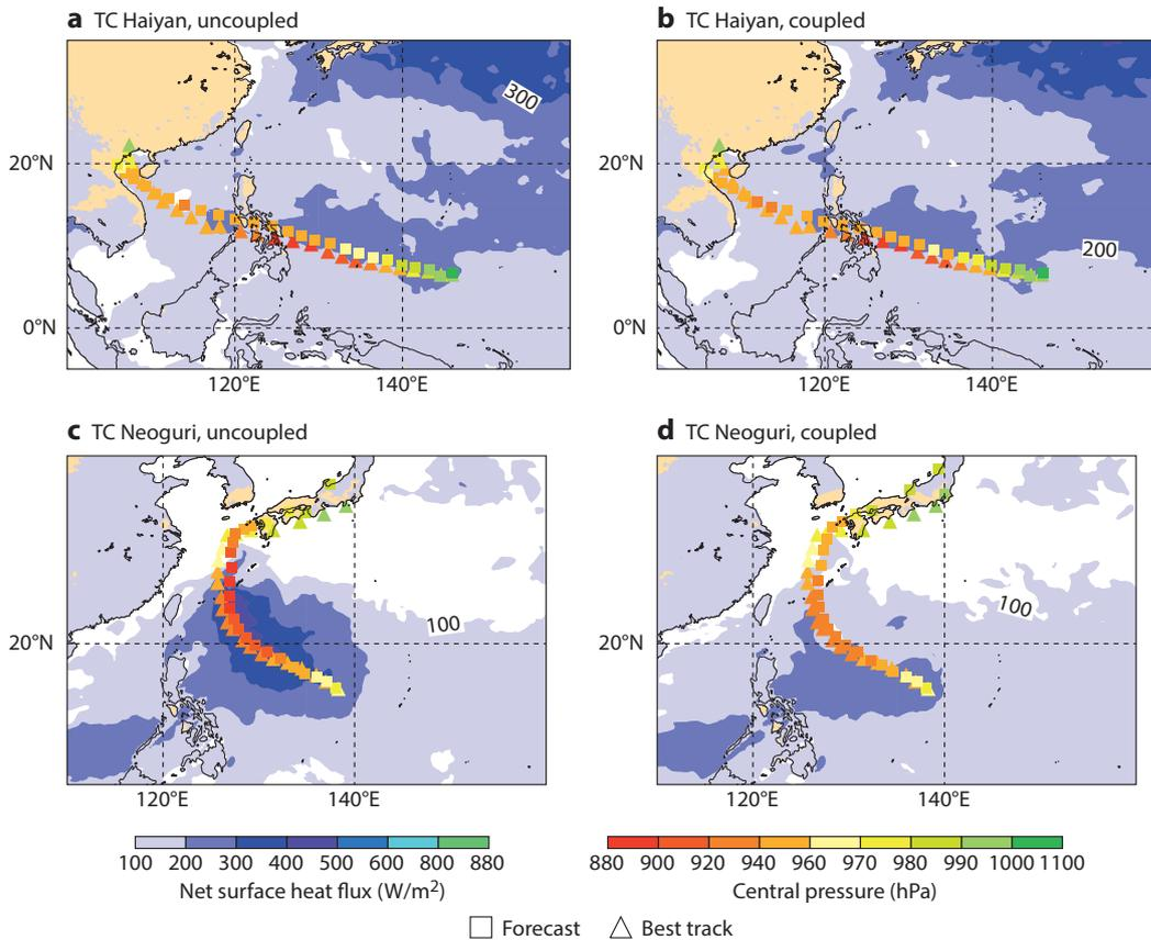
**Figure 1** The plots show five-day HRES track and intensity forecasts (squares) together with ‘best track’ estimates (triangles) and the predicted net surface heat flux (shading) for (a) TC Haiyan (starting date 5 November 2013) using the uncoupled model, (b) TC Haiyan using the coupled model, (c) TC Neoguri (starting date 5 July 2014) using the uncoupled model, and (d) TC Neoguri using the coupled model.
