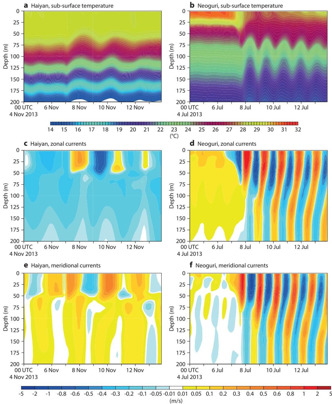
**Figure 5** Plots of sub-surface temperature and currents for the two points on the model track closest to the estimated Haiyan ‘best track’ position at 00 UTC on 7 November 2013 and for Neoguri at 18 UTC on 7 July 2014, showing ocean forecasts of (a) sub-surface temperature for Haiyan, (b) sub-surface temperature for Neoguri, (c) zonal (east–west) currents for Haiyan, (d) zonal currents for Neoguri, (e) meridional (north–south) currents for Haiyan, and (f) meridional currents for Neoguri.
