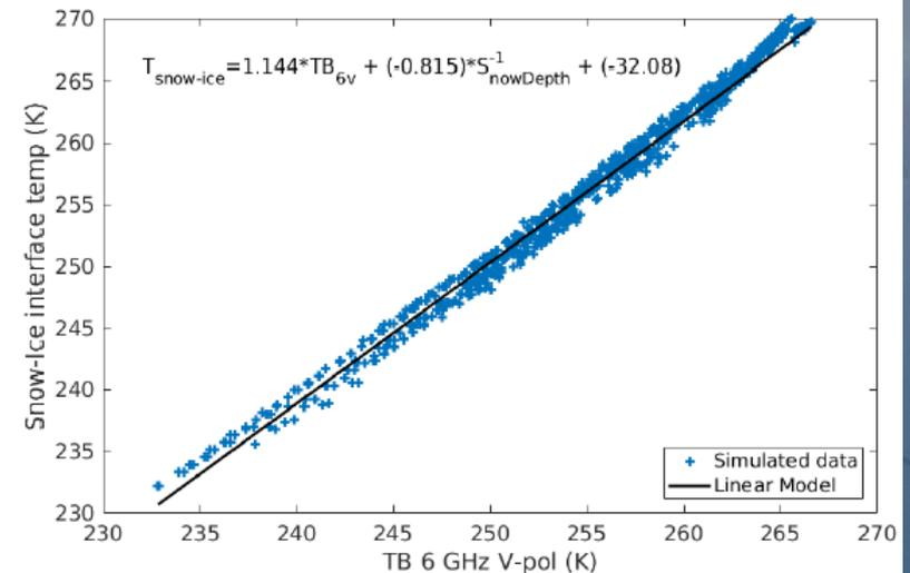
Figure 15: Snow ice interface temperature from memls data as a function of the brightness temperature at 6.9 GHz in blue points, and the multi-linear regression for the mean snow depth in black line.
