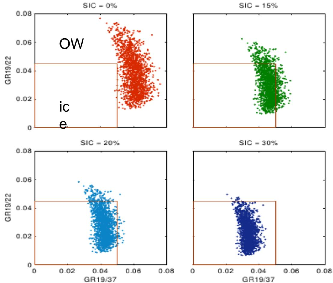
**Figure 5.** Demonstration of the open water/weather filter performance: gradient ratio (GR) 19/22 is plotted as a function of GR19/37 for SSM/I data in 2008 (entire year) for the Northern Hemisphere for sea ice concentration (SIC) of 0, 15, 20, and 30%. The red square shows the value range outside which the open water/weather filter sets SIC values to 0% (open water).
