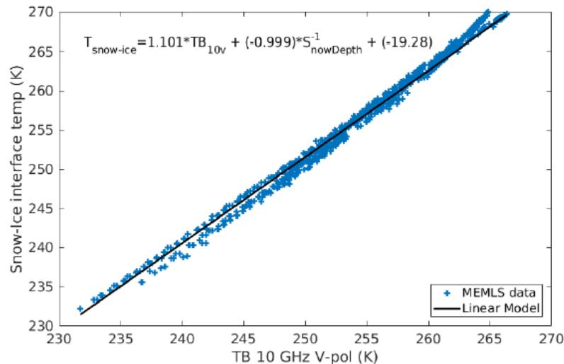
Figure 14: Snow ice interface temperature from memls data as a function of the brightness temperature at 10.65 GHz in blue points, and the multi-linear regression for the mean snow depth in black line.
