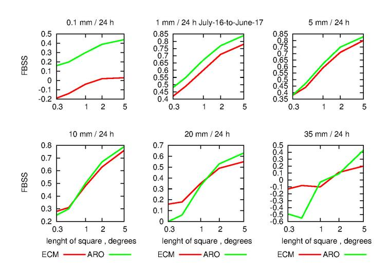
Figure 3: FBSS for different thresholds of precipitation. FBSS at the vertical axis and the size of different squares in degrees. There should be at least three observations in a square for being used in the verification. One degree is about 111 km. ECM (red) is ECMWF forecasts and ARO (green) is AROME with 2.5 km grid.
