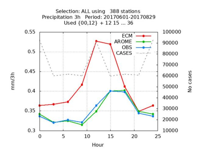
Figure 2: Diurnal cycle of 3-hour precipitation. Hours of the day on horizontal axis, precipitation on vertical axis. Red: ECMWF, green: AROME and blue observations. Area: North-western Europe. Time period : June-August 2017. Forecast lengths: 12, 15, 18, 21, 24, 27, 30, 33 and 36 hours.
