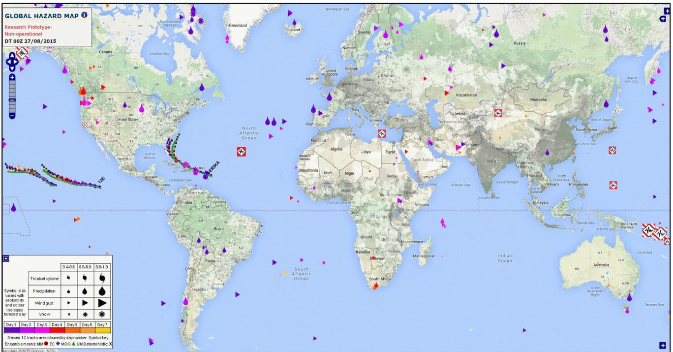
Fig.6 GHM symbol-based summary map showing an 'at-a-glance' view of forecast high-impact weather for the week ahead. Symbols are sized based on probability and coloured based on lead time.
