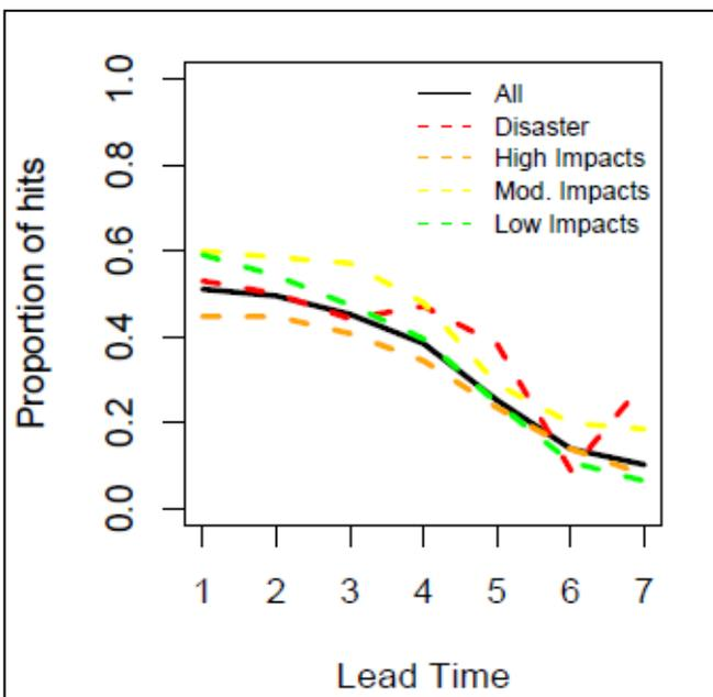
Fig.9 Plot illustrating the proportion of hits obtained by comparing intersects between heavy rainfall impact polygons and GHM forecast precipitation summary polygons, for matching occurrence ('observed') and validity ('forecast') dates. Results are split based on the impact severity of each impact record.
