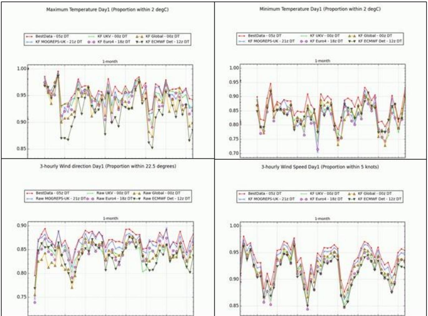
Fig.3 A selection of monthly verification statistics for Day 1 surface parameters used to create the BestData blend. The ECMWF HRES forecast is used in the blend. KF=Kalman Filter.
