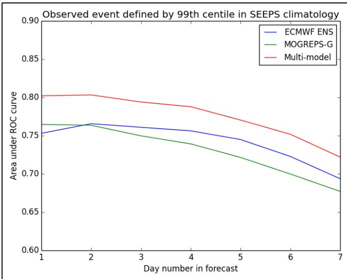
Fig.8 Area under the ROC curve for the three ensemble forecast models for 24-hour precipitation exceeding the 99th percentile of the M-Climate climatology for each day in the forecast. Verification is carried out against station-based observations at 3315 sites for the period 4th February 2015 - 31st December 2015, with the observed event defined by the 99th percentile in the SEEPS climatology.
