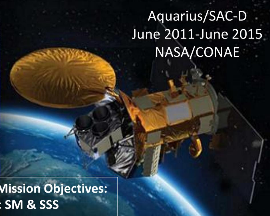
The image shows the Aquarius/Satellite Application of Ocean Color Dynamics (SAC-D) satellite. It features a large, circular, gold-colored antenna dish and various instruments on its body. The Earth is visible below.
