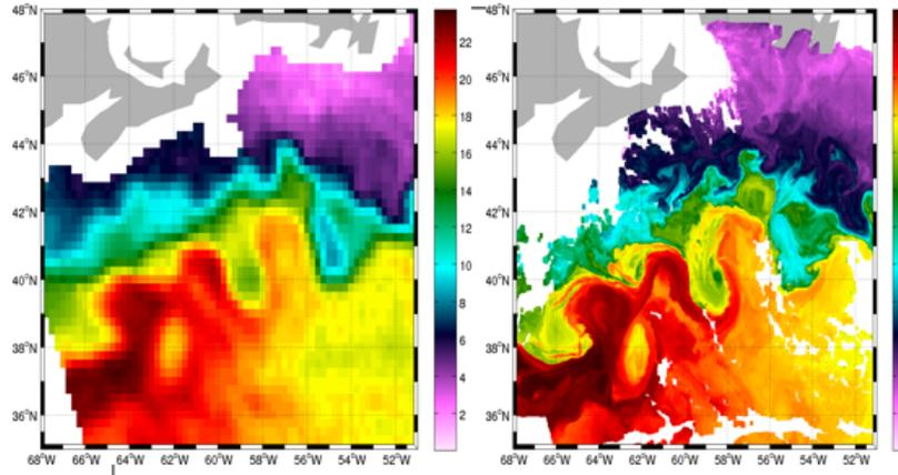
Microwave (MW) and infrared (IR) from SSTs AMSR-E and MODIS
