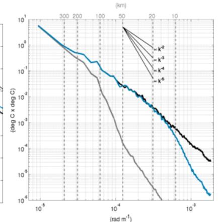
Left : Reconstructed HR SST field from the AMSR-E data ; Middle : example of SST front from AMSR-E (grey), MODIS (black) and the reconstructed field (blue). Right : SST spectra from AMSR-E (grey), MODIS (black) and the reconstructed field (blue).
