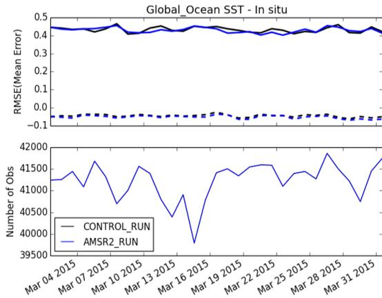
Global Ocean SST errors in the Control experiment (black) and in AMSR2 experiment (blue)
