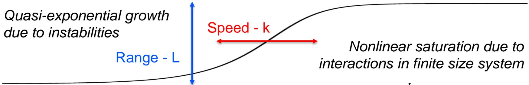
The standard logistic function is the logistic function with parameters ( $k = 1$ ,  $x_0 = 0$ ,  $L = 1$ ) which yields
