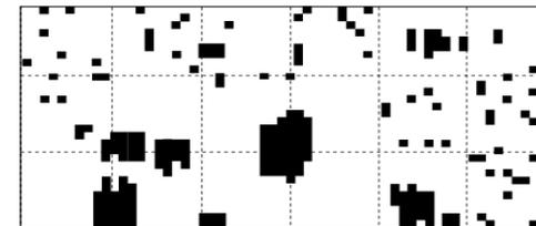
Probability of an "on" cell proportional to CAPE and number of adjacent "on" cells – "on" cells feedback to the resolved flow
