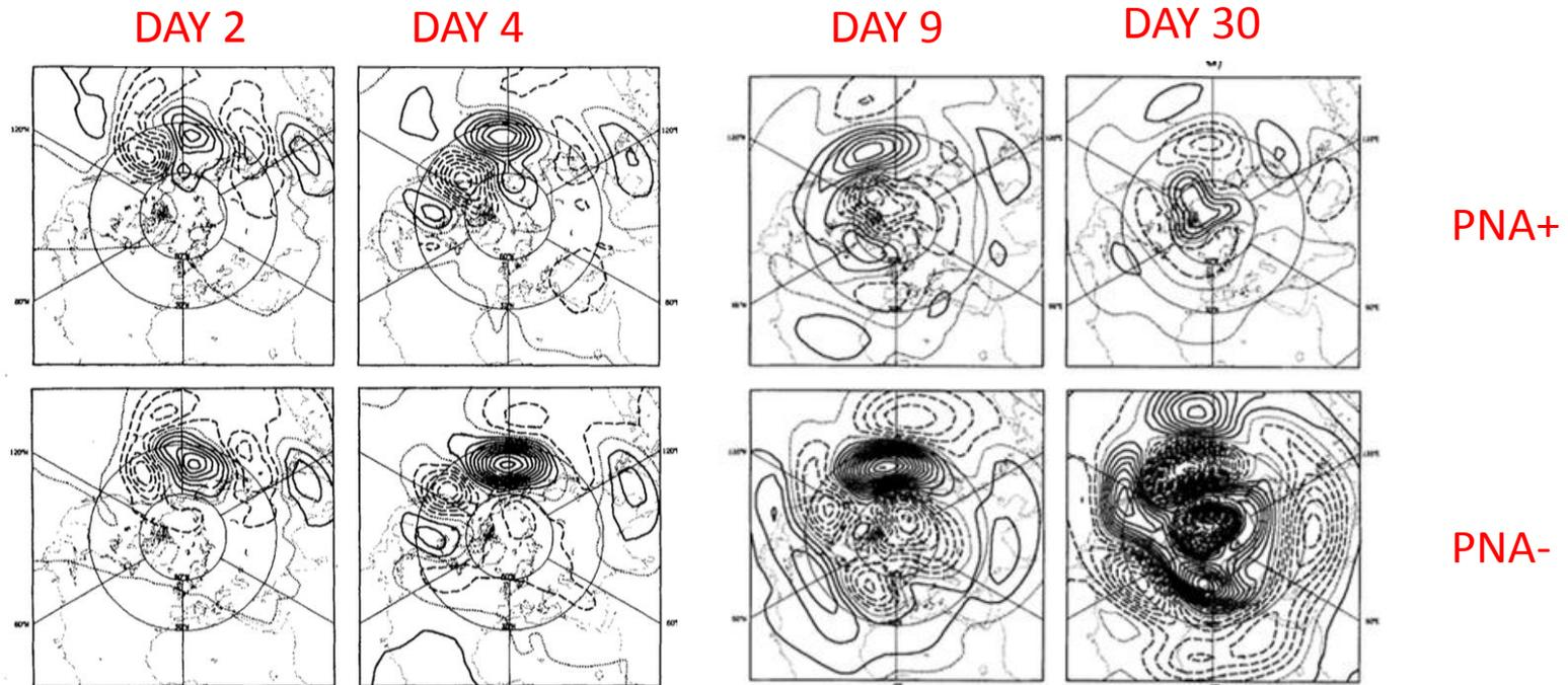
Figure 9. Perturbation streamfunction from integrations of a barotropic model with the two basic states shown in Fig. 8, and identical perturbations positioned at 30°N 120°E. The top diagrams are for basic state B-, the bottom for B+. (a) Day 2; (b) day 4; (c) day 9; (d) day 30. For details see text and Simmons *et al.* (1983). The
