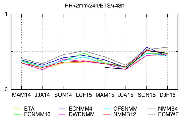
Fig.17-18 FBI and ETS of ECMWF 24h precipitation forecast (48h) for seasons MAM14 to DJF16. Threshold is 2mm/24h. Comparison to operational NWP models forecast.
