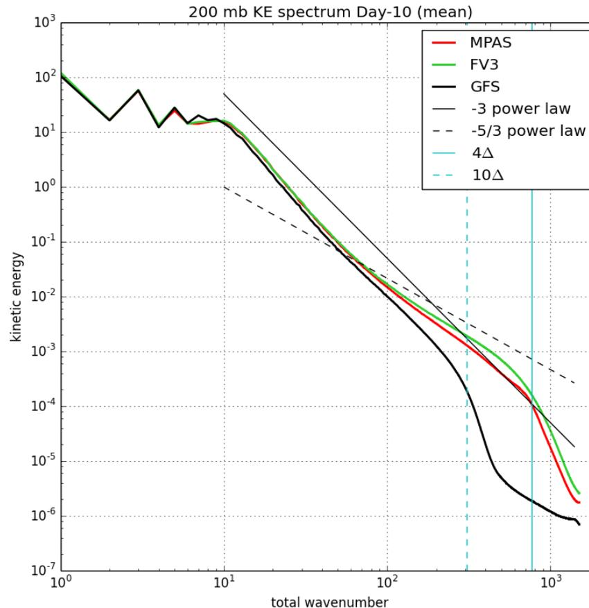
**Figure 3.2:** 10-day forecast 200 hPa kinetic energy (KE) spectra, averaged over all 74 forecasts. Reference power-law spectra corresponding to powers of -3 and -5/3 are shown for reference, as well as scales corresponding to 4 and 10 times the nominal grid resolution.
