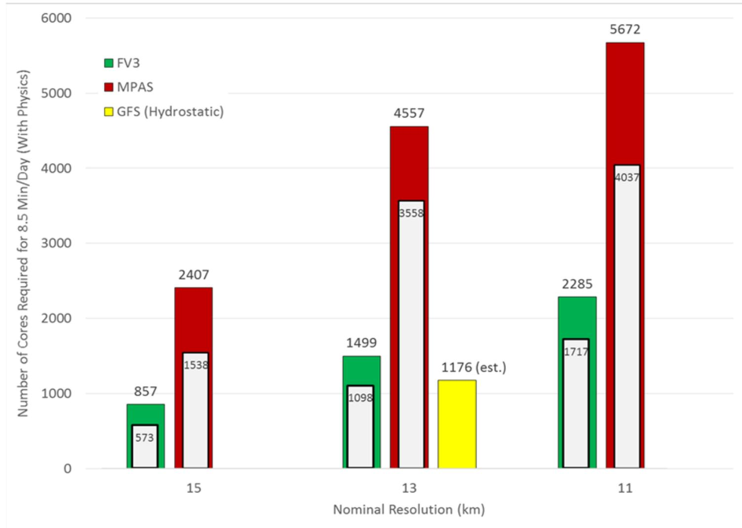
Figure 2: Cores required to meeting 8.5 minutes per day forecast speed requirement for operations at 15, 13, and 11 km horizontal resolution. All cases used 63 vertical levels. Colored bars show time with GFS physics; insets show the fraction of cores required by the dycore alone. The estimated number of cores required to run the 13 km operational GFS in 8.5 minutes on NCEP's WCOSS Cray XC40 is shown for comparison.
