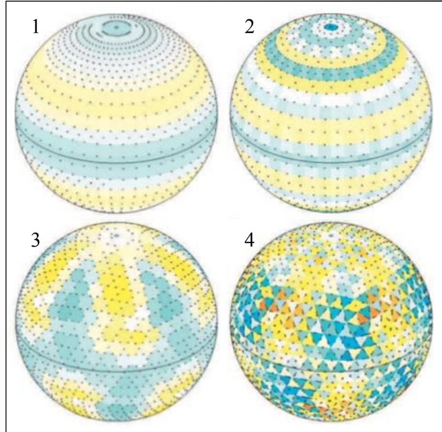
**RIGHT:** Figure shows relative height errors for nonlinear SWE's: 1. lat-lon grid. 2. lat-lon with “skipped” nodes at high latitudes. 3. hexagonal icosahedron. 4. triangular icosahedron (geodesic). Study used unstructured C-grid model TRiSK. (Weller et.al, JCP 2012.)
