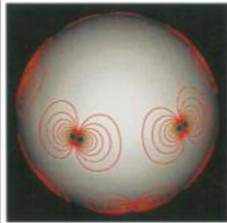
Geodesic Grid, “spring” grid divergence error, (Tomita et.al, JCP 2001) + Lambert conformal mapping (Iga and Tomita, JCP 2014)
