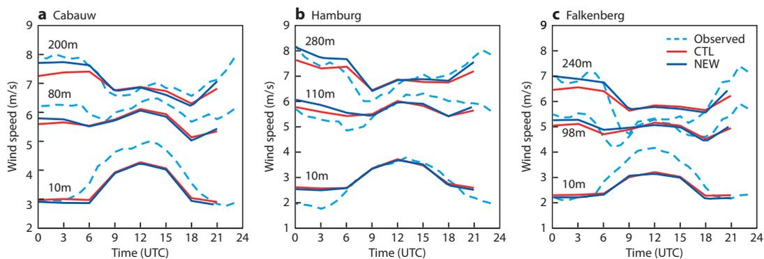
**Figure 3** Averaged diurnal cycle of wind at (a) Cabauw, (b) Hamburg and (c) Falkenberg from forecasts produced in the CTL and NEW experiments (lead times 24 to 42 hours) compared to observations. Note that for Falkenberg the jump around 100 metres is due to the data below 100 metres coming from tower measurements and above 80 metres from sodar. Results are shown for June to August when the diurnal cycles are the most pronounced.
