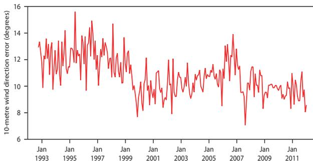
**Figure 1** Historic evolution of 10-m wind direction errors of the IFS. These are monthly values of mean errors at a lead time of 60 hours of the daily forecasts initialized at 12 UTC (verifying time 00 UTC). The verification includes 800 SYNOP stations over Europe (30°–72°N, 22°W–42°E).
