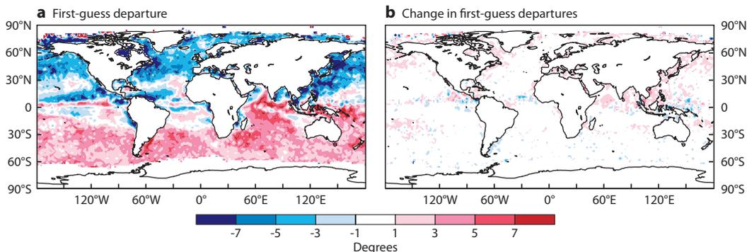
**Figure 2** (a) Mean first-guess departure (observations minus model) of wind direction at the surface (degrees) with respect to ASCAT scatterometer observations in the CTL analysis run and (b) the mean change in these first-guess departures in the NEW experiment with respect to the CTL. These quantities represent the average over the 00 and 12 UTC analyses. Results shown here are for June to August when the stable regions over the oceans are more extended than in January to March.
