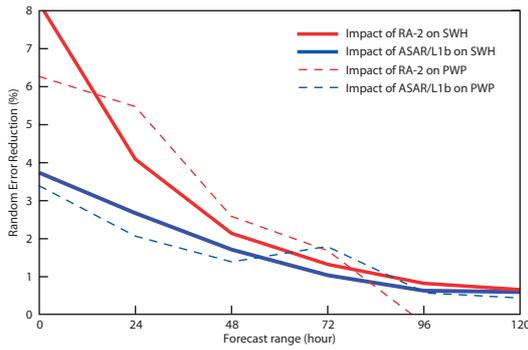
**Figure 3** Random error reduction (%) in the tropics against buoys as function of the forecast day and computed for either Exp/ASAR or Exp/RA2 with respect to Exp/Base during the period 1 January to 31 March 2012. The impact is shown for significant wave height (SWH) and the peak wave period (PWP).
