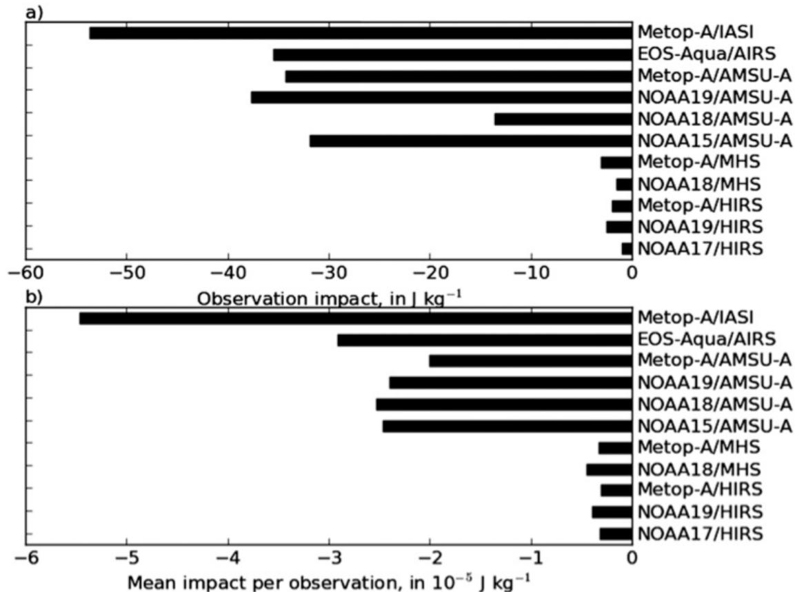
FIG. 5. (a) Observation impact and (b) mean impact per observation of the instruments using MWS and IRS techniques.
