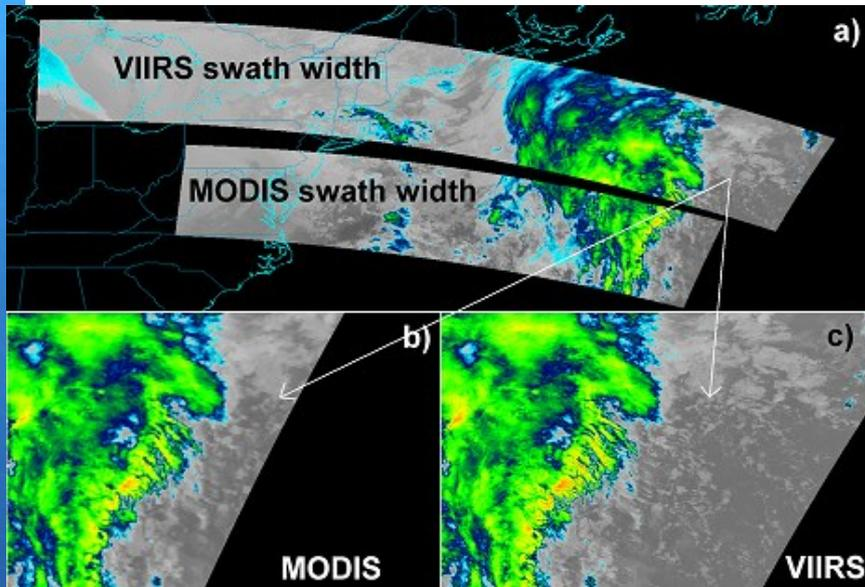
The Visible Infrared Imaging Radiometer Suite offers more spectral bands, higher resolution, wider swath and greater accuracy, resulting in a large number of products.
