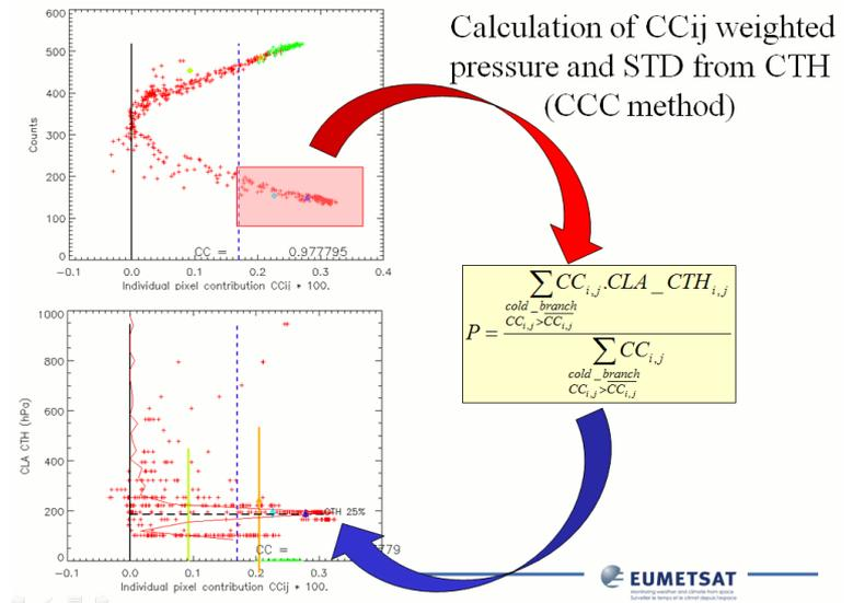
Pixel contribution to the cross correlation coefficient, CCij, is used to select the pixels that contribute most to the tracking
