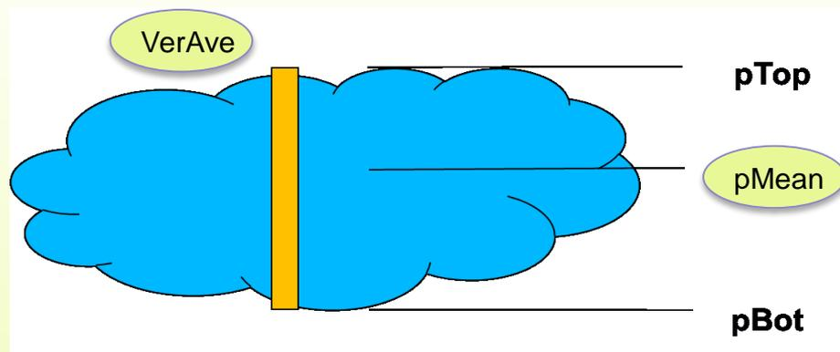
**pMean** – weighed mean of model levels within the cloud, weights proportional to ice (or liquid water) content.
