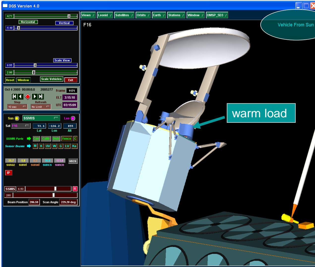
For F-16 - 3 or 4 times per orbit solar radiation illuminates warm load tines, through:
