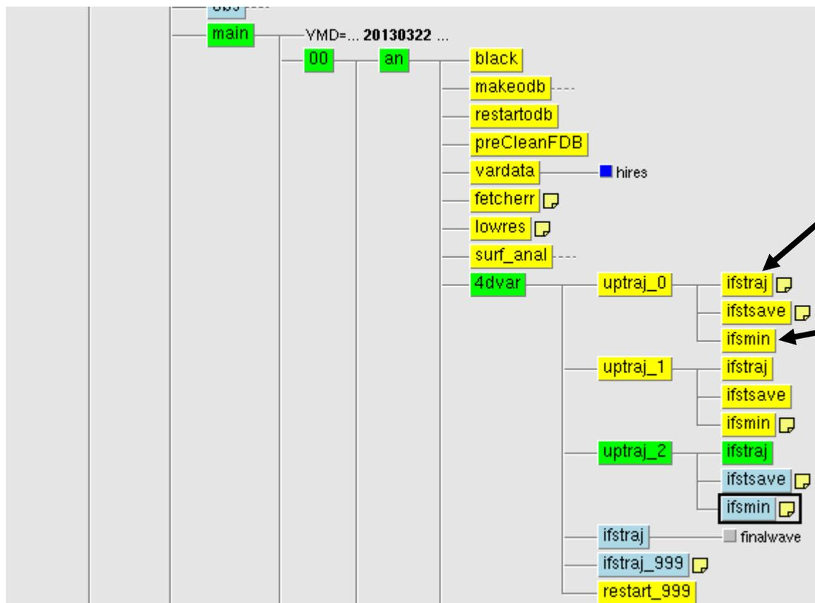
We use the full non-linear operators here in the “trajectory runs”. This is the “**Outer loop**”.
