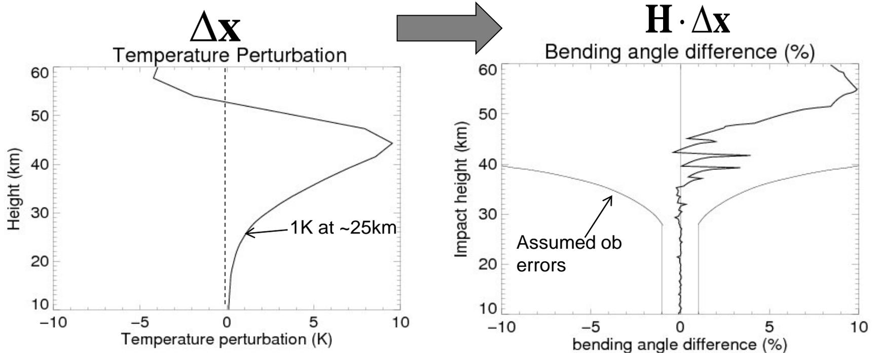
The null space arises because the measurements are sensitive to  $\sim P(z)/T(z)$ . *A priori* information is required to split this into  $T(z)$  and  $P(z)$ .
