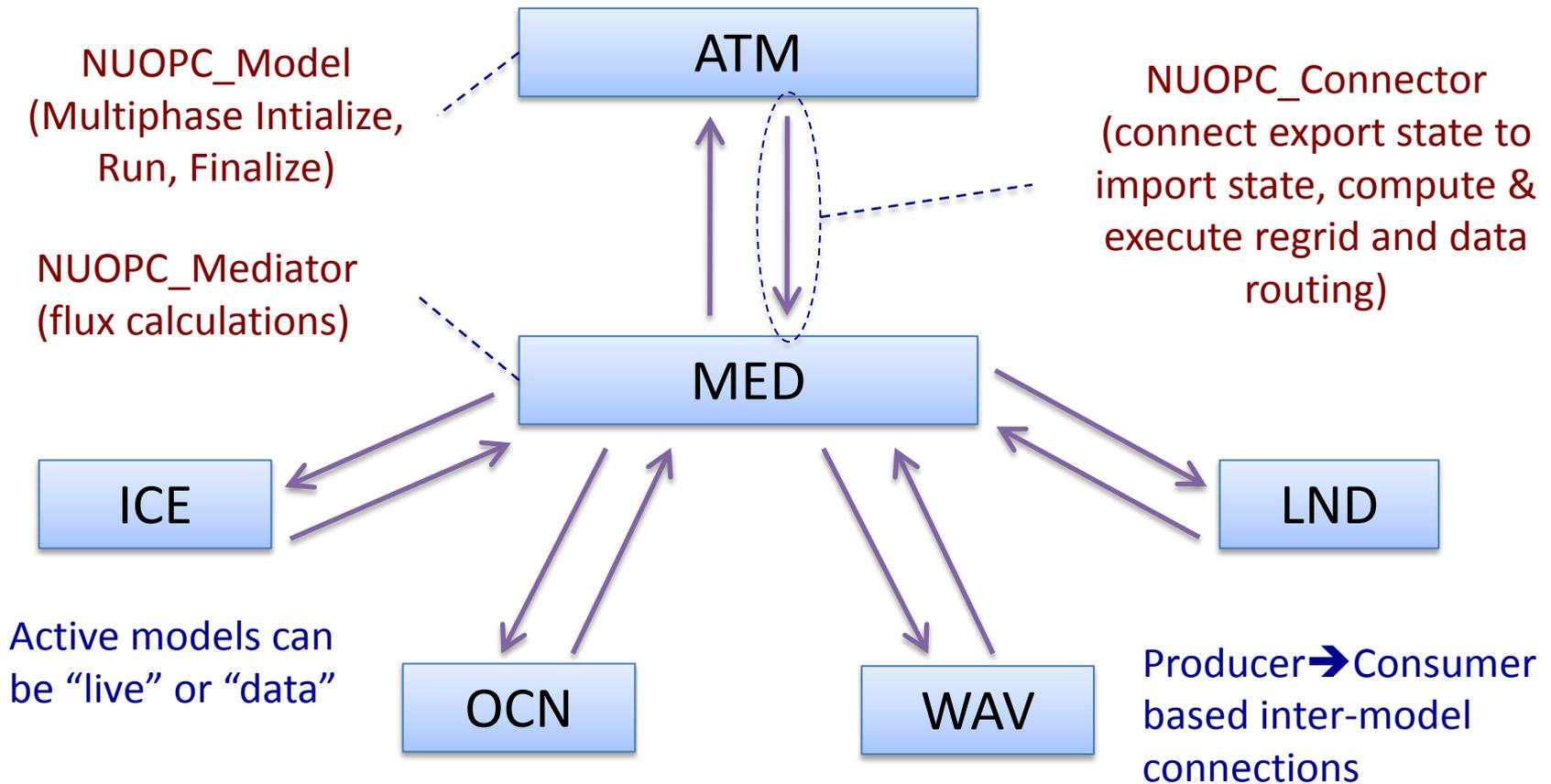
ESMF/NUOPC interface layer is being implemented into each of the Navy relevant models (NAVGEM, HYCOM, WWIII, CICE). ESMF/NUOPC based coupling infrastructure integrates the models, together with a flux exchange layer, into a flexible coupled system.
