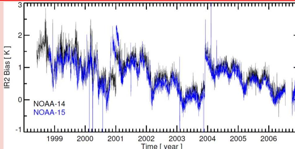
*Fig: Time series of Meteosat-7 infra-red biases relative to HIRS/2 from NOAA-14 and NOAA-15*
