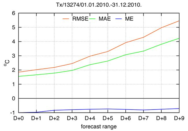
**Figures 1–2** ME, MAE and RMSE of ECMWF 2 meter minimum and maximum temperature forecast (D+0 to D+9) as a function of forecast range (Beograd - Karađorđev park).
