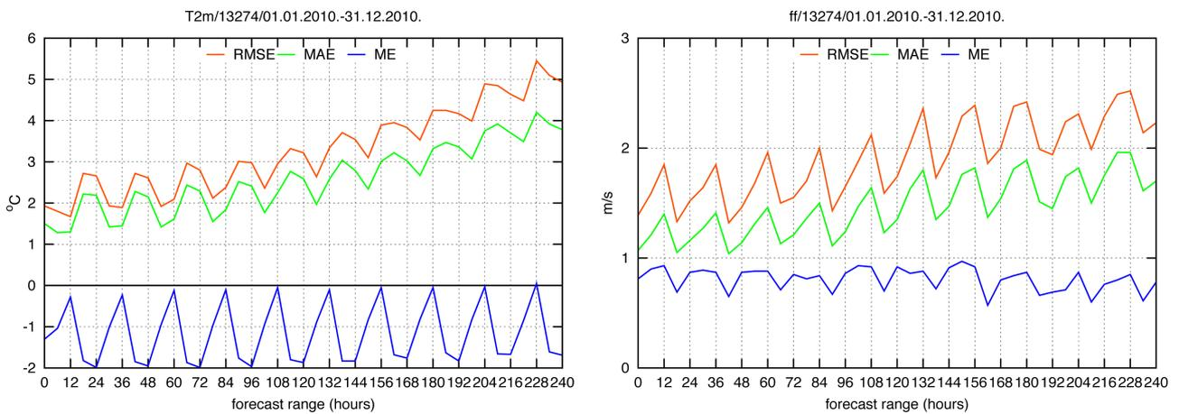
**Figures 7–8** ME, MAE and RMSE of ECMWF 2 meter temperature and 10 meter wind speed forecast as a function of forecast range (Beograd - Karađorđev park).
