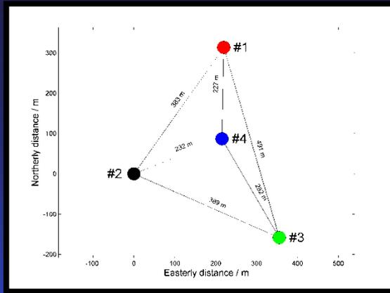
An array of four microbarographs with a sensitivity of 0.1Pa, buried  $\sim$ 1 m below the porous firn surface and sampled at 0.1Hz. Mean array distance c. 300 m.
