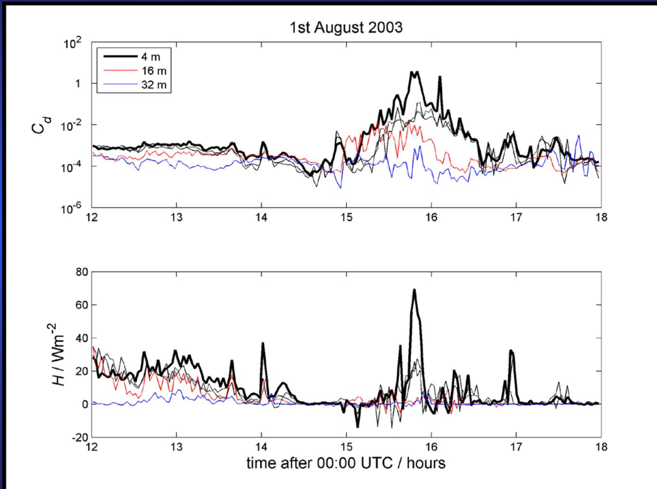
Example of a burst of turbulence in stable, near calm conditions resulting in a >100-fold increase in drag coefficient and large pulse downward of sensible heat flux
