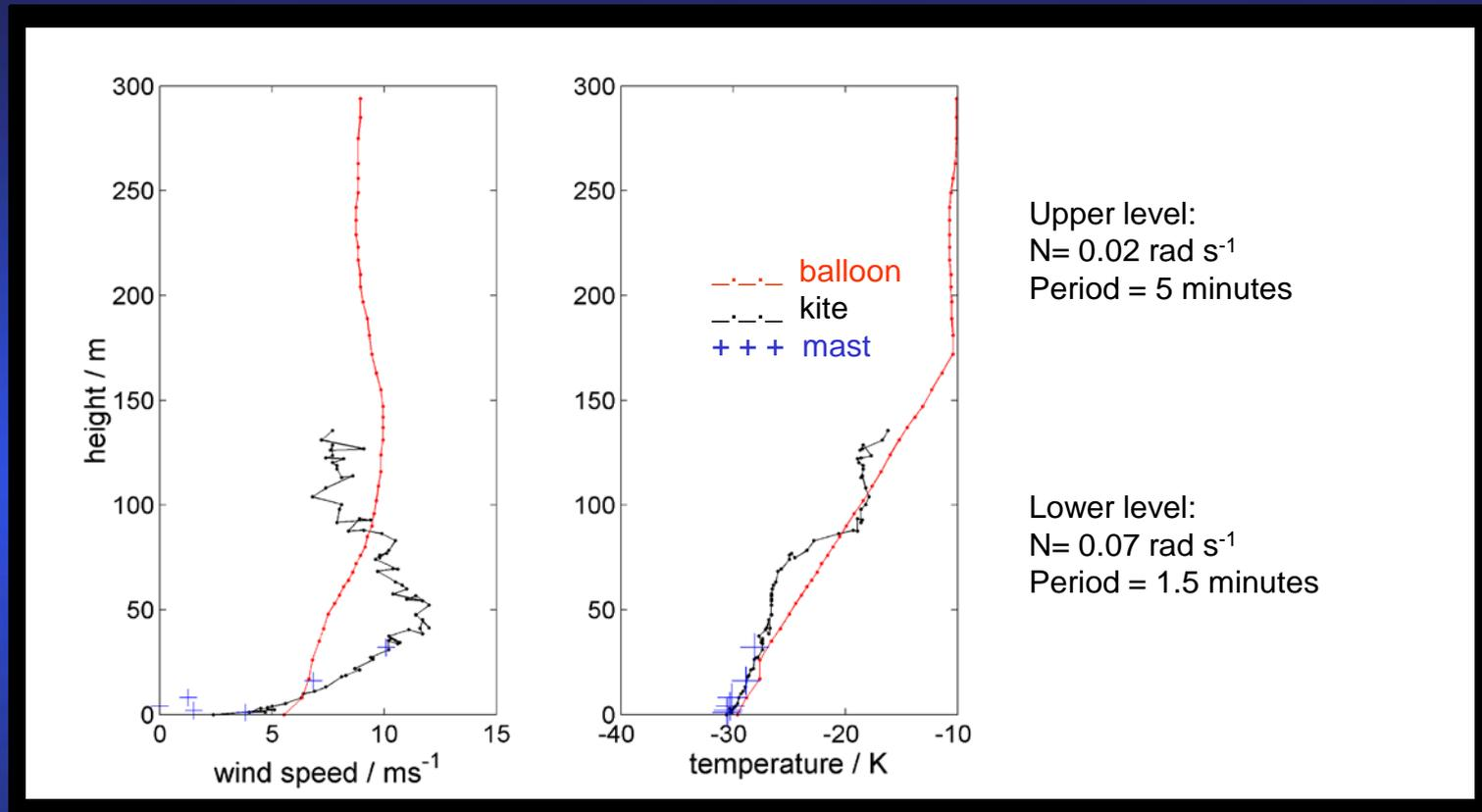
Comparison of radiosonde, kite and mast platform instruments: structure is smoothed out in the radiosonde, but likelihood that the upper levels tend to isothermal regime. Parameterisation on upper level  $N$  will therefore be invariant.
