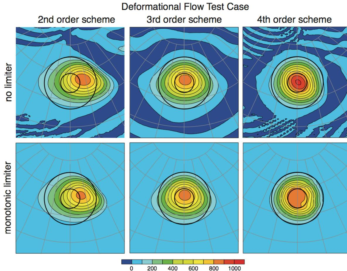
FIG. 5. Deformational flow test case results at time  $T$ . The thick contours are the exact solution for  $\psi = 100$  and  $800$ . The simulations were performed on the 40962-cell grid.
