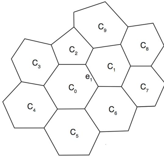
Edge  $e_1$  has weights for computing second derivatives at cell centers  $C_0$  and  $C_1$ .
