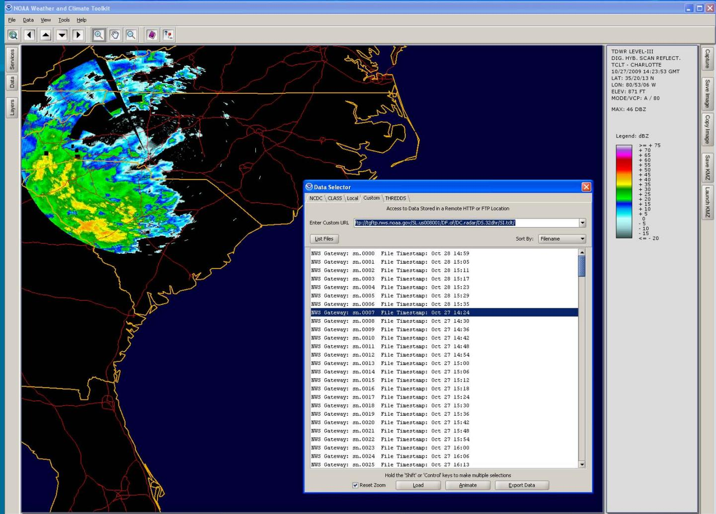
TDWR data displayed in toolkit using near real time data accessed from NWS server
