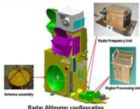
Radar Altimeter configuration
