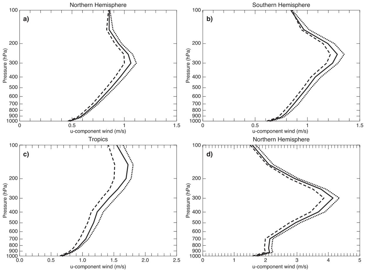
Figure 6: R.m.s. east-west wind component ensemble spread, or forecast error, ( $\text{ms}^{-1}$ ), for (a) the extratropical Northern Hemisphere, (b) Southern Hemisphere, and (c) the tropics, at 12-hours, and (d) for the Northern Hemisphere at 120 hours, for each of the three experiments: Control (full line), NoSonde (dotted) and ADM-Aeolus (dashed). Note the scale runs from 0 to 1.5 in (a) and (b), to 2.5 in (c) and to  $5.0 \text{ms}^{-1}$  in (d).
