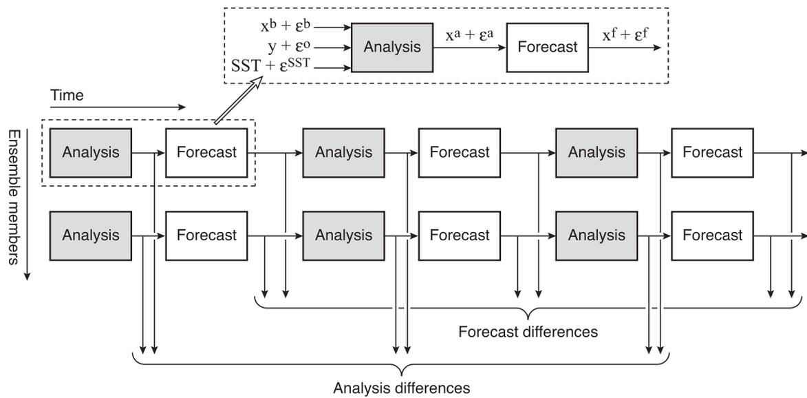
Figure 2: Ensemble of data assimilation cycles, schematic. See main text for definitions.
