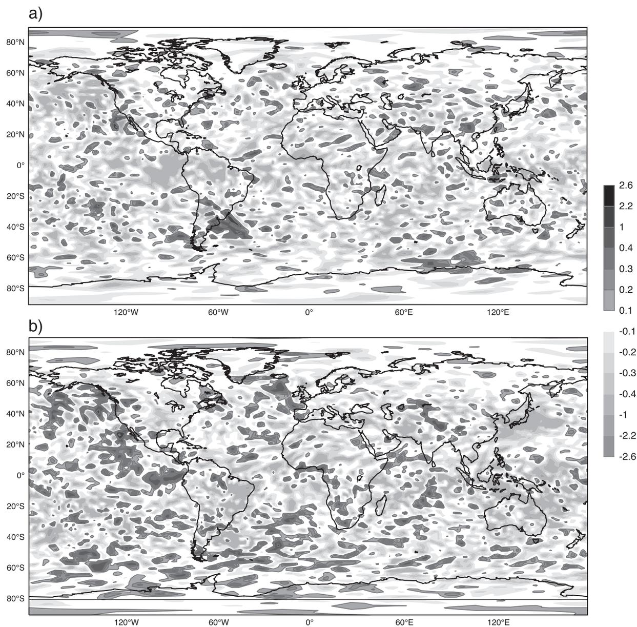
Figure 5: Impact in terms of 300 hPa zonal wind component ( $\text{ms}^{-1}$ ) of (a) ADM-Aeolus wind profile data and (b) Sonda data, as deduced from the difference in 12 hour forecast spread between ensembles. Light (dark) grey shading (see legend) indicates that the ensemble spread, i.e. the analysis error, is reduced (increased) using the data. Shading in the range  $-0.1$  to  $0.1 \text{ms}^{-1}$  is suppressed.
