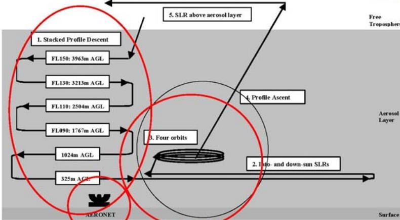
**Figure 2:** Schematic diagram of the flight pattern performed by the C-130 over the Etosha AERONET site on September 13, 2000. Consisting of 1) stacked profile descent, 2) into- and down-sun SLRs, 3) a series of four orbits, 4) profile ascent, 5) SLR above the aerosol layer.
