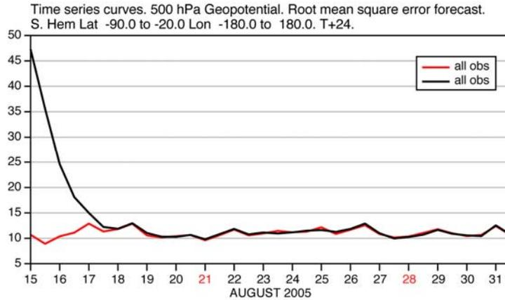
Figure 2: RMS 24-hour forecast scores for southern-hemisphere geopotential at 500hPa for two runs of the analysis-forecast system, differing only in the initial background state.
