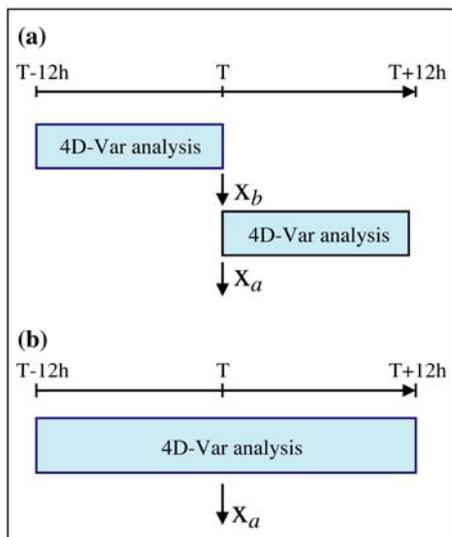
Figure 1: (a) Schematic showing a pair of consecutive 4dVar analyses with 12-hour analysis windows, and with the analysis time defined to coincide with the start of the analysis window. (b) An alternative configuration with a 24-hour window.
