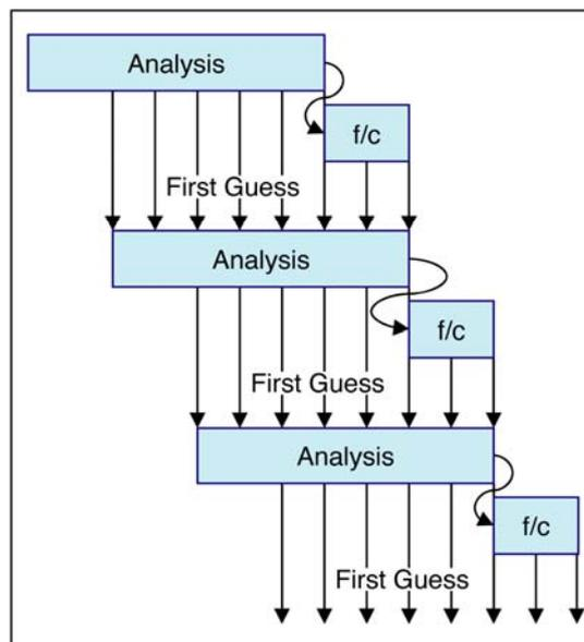
Figure 3: Schematic showing the cycling of overlapping analysis windows. “f/c” indicates a short forecast initialized at the end of the preceding analysis window.
