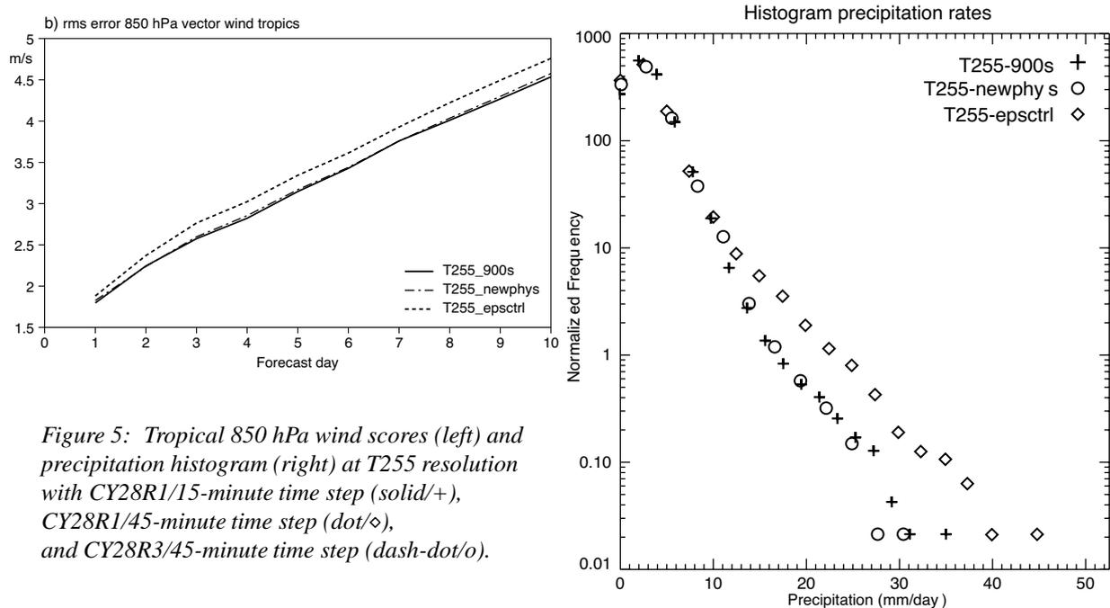
Figure 5: Tropical 850 hPa wind scores (left) and precipitation histogram (right) at T255 resolution with CY28R1/15-minute time step (solid/+), CY28R1/45-minute time step (dot/d), and CY28R3/45-minute time step (dash-dot/o).
