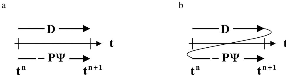
Figure 1: Parallel time splitting (a) and sequential time splitting (b).  $D$  represents the dynamics tendency and  $-P\Psi$  represents the physics tendency.
