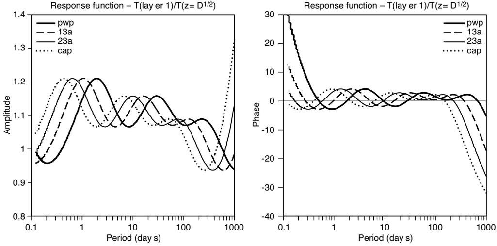
Figure 10: Error in amplitude and phase of the discretized soil temperature equations with layer depths of 7, 21, 72 and 189 cm. Four different constant diffusion coefficients are used corresponding to the soil moisture range from permanent wilting point to field capacity.
