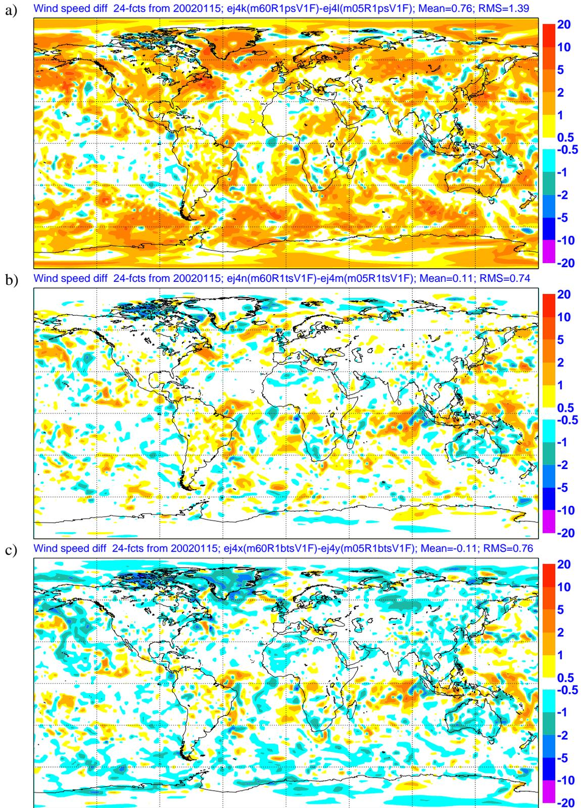
Figure 2: Wind speed (10 m) time truncation errors of a 24 hour forecasts with a 60 minute time step with different time stepping procedures for the vertical diffusion scheme: (a) parallel splitting (b) sequential splitting and (c) sequential splitting but the diffusion coefficients are computed after the dynamics increments have been added. An integration with a 5 minute time step is used as a reference (differences between schemes with 5 minute time steps are small).
