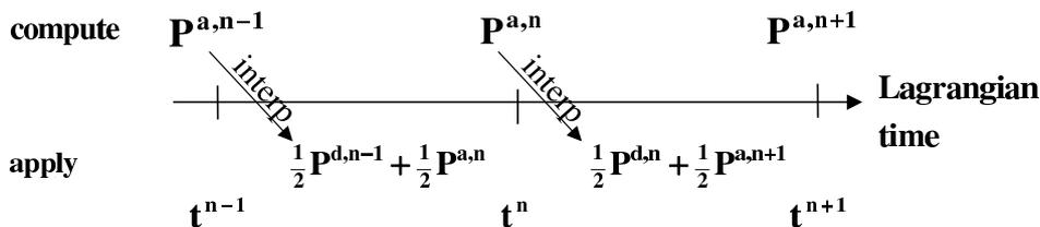
Figure 3: Schematic of Semi-Lagrangian Averaging of Physical Parametrizations (SLAVEPP).  $P$  represents the physics tendency.
