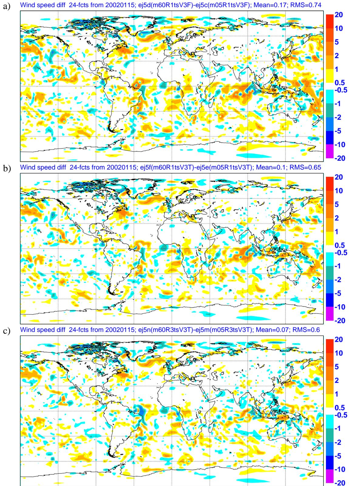
Figure 4: Wind speed (10 m) time truncation errors of 24 hour forecasts with a 60 minute time step with (a) standard time stepping (b) SLAVEPP as in CY28R1 and (c) revised SLAVEPP as in CY28R3 with an additional call to the cloud scheme before convection. An integration with a 5 minute time step is used as the reference.
