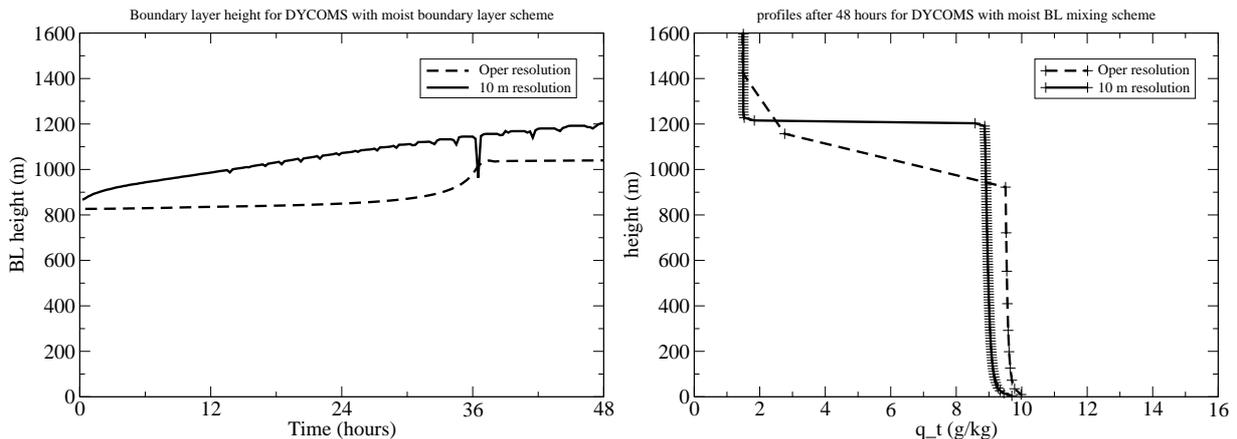
Figure 8: Time evolution of inversion height (left figure) and vertical profile of specific humidity (right figure) from single column simulations with the ECMWF model of a stratocumulus case with operational resolution (typically 200 m at inversion height, dashed) and 10 m resolution (solid).
