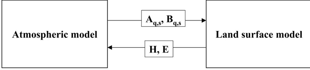
Figure 11: Exchange of parameters between atmospheric models and land surface schemes for universal coupling (Best et al. 2004).
