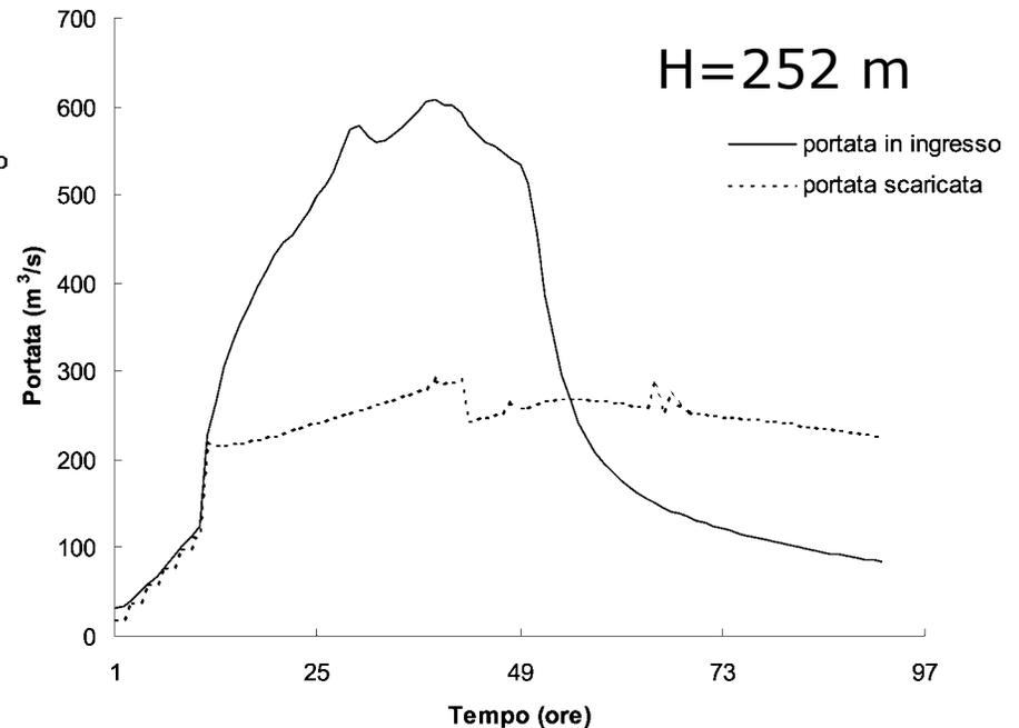
An improvement is observed when optimized gate operations are introduced: the availability of additional volumes in the reservoir, obtained by lowering the level in the lake before the flood allows the safe containment of the 50yrs flood event
