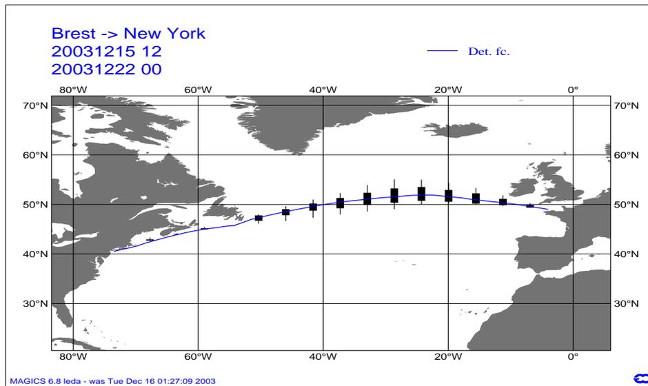
Figure 2: Example of ship route forecast for the route between Brest and New-York in a case where the ensemble spread is relatively large. The plot shows the deterministic forecast (blue line) and the ensemble forecast (error bars). The boxes show the 10 and 90 percentiles for the spread of the ship routes, and the whiskers depict the positions of the outliers. The forecasts starts at 12Z 15th December 2003.
