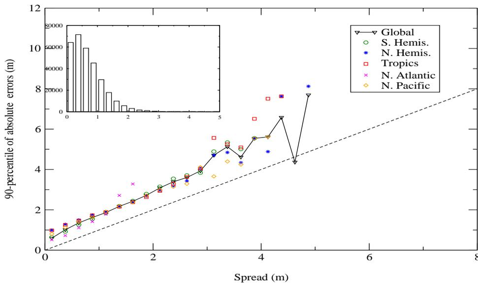
Figure 3: The spread-skill relationship for waves. The plot is based on global altimeter observations. The black solid line is the result when all data are used. The symbols show the result when the data are divided into different areas. For reference, the black dashed line shows the 45 degree diagonal. The bar diagram in the upper left corner gives the number of observations in each bin.
