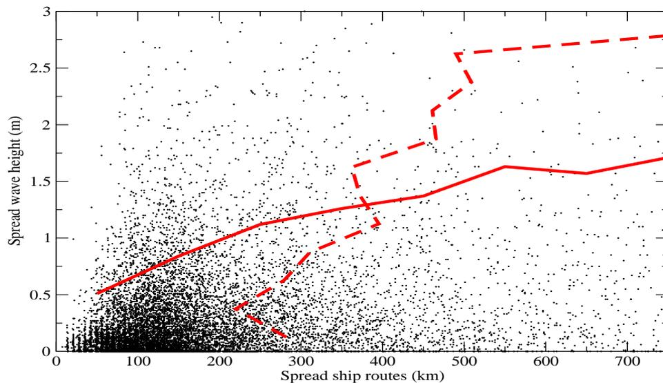
Figure 4: Relationship between the spread of the ensemble waves and the ensemble ship routes. The black dots represent the data pairs. The red solid line is the 90 percentile of the wave spread in the ship spread bins and the red dashed line is the 90 percentile of the ship spread in wave spread bins.
