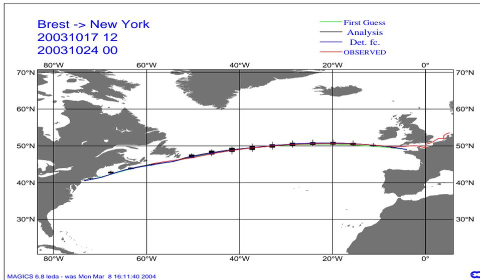
Figure 1: Ship routes for the crossing between Brest and New-York. The plot shows the deterministic forecast (blue line), The first guess (green line), the analysis (black line), the ensemble forecast (error bars). The boxes show the 10 and 90 percentiles for the spread of the ship routes, and the whiskers depict the positions of the outliers. The red line is the route used by the container vessel Leverkusen Express. The forecasts start at 12Z 14th October 2003.
