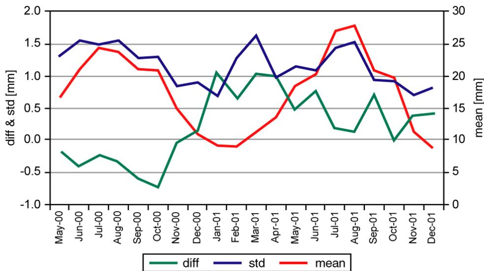
Figure 3: Monthly statistic of GPS PW (station LDBG) minus co-located radiosonde PW Lindenberg from May 2000 to December 2001: mean difference GPS PW minus radiosonde PW (diff), standard deviation of the difference (std) and mean GPS PW (mean).
