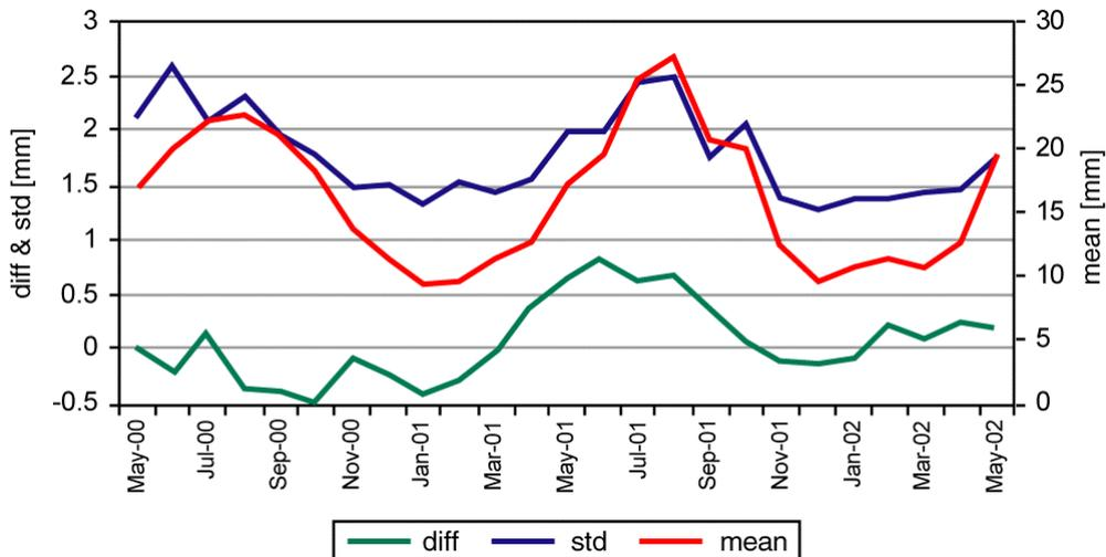
Figure 2: Monthly statistics of GPS PW minus LM PW (operational assimilation fields) over 23 stations, from May 2000 to May 2002: mean difference GPS PW minus LM PW (diff), standard deviation of the difference (std) and mean GPS PW (mean).
