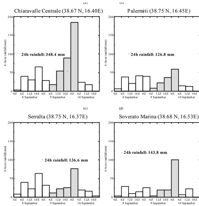
Figure 2 Soverato case. Observed values of precipitation, accumulated every 6 hours in four stations in the vicinity of the areas flooded during the “Soverato flood”. The position of the station is indicated on the top of each panel, while the 24-hour cumulated precipitation relative to the 9<sup>th</sup> of September (grey bars) is reported in the panel.
