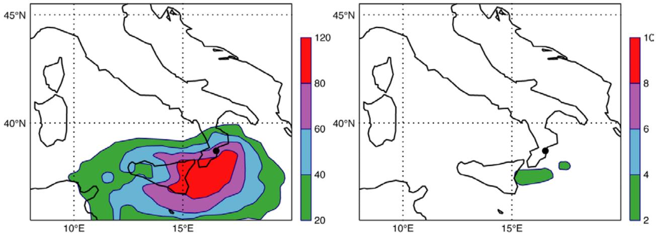
Figure 3 - Soverato case. Probability maps of precipitation exceeding 20mm/day (left panel) and 50mm/day (right panel) relative to the most recent global ensemble EPS (60-hour forecast range, model used T255). The black dot denotes the approximate location of Soverato (38.68°N, 16.55°E).
