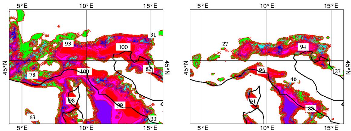
Figure 9 MAP IOP2b case. Probability maps of precipitation exceeding 20mm/day (left) and 50mm/day (right) relative to the 5-member LEPS using the non-hydrostatic model Lokal Modell at 7 Km horizontal resolution. Contour interval every 10%.
