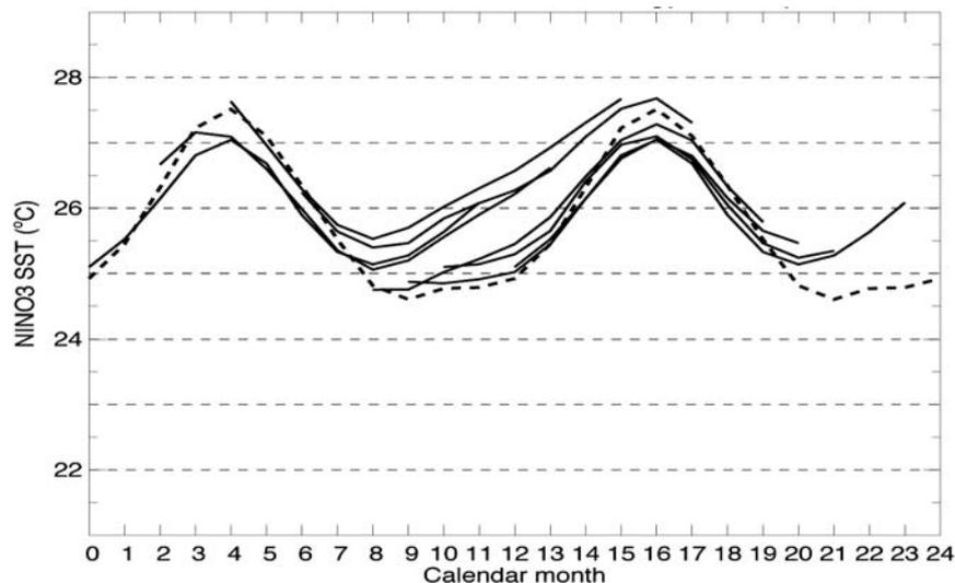
Figure 2: Climatological drift of Niño-3 SST as a function of forecast start month. The drift is calculated from 6-member ensemble forecasts conducted for a duration of 12 months from 1993 to 2001. The dashed line is a climatology of Reynolds SST calculated over the same time period.
