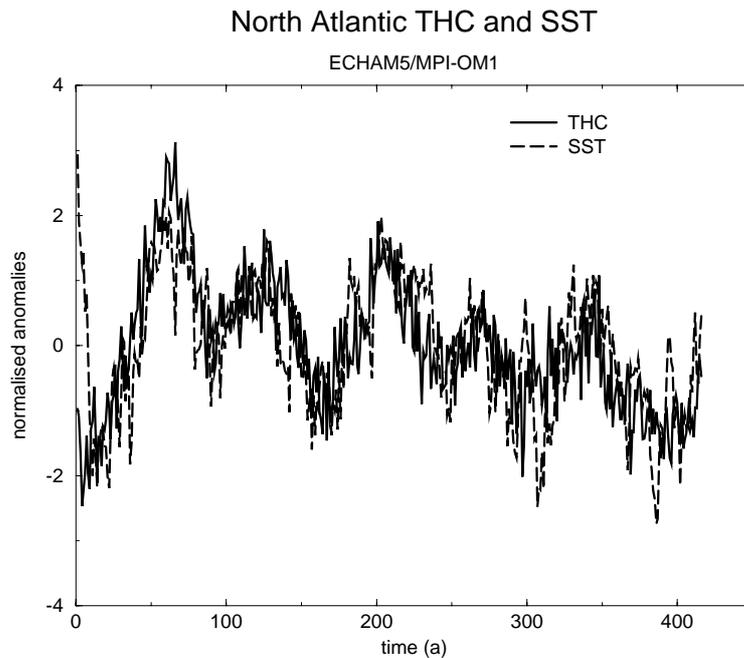
*Figure 2: Time series of simulated annual mean North Atlantic SST anomalies (40-60°N and 50-10°W, dashed line) and annual mean anomalies of the maximum overturning at 30°N (full line), a measure of the strength of the model's thermohaline circulation. Note that both time series are highly correlated at timescales beyond several years indicating that the low-frequency variations of the THC can be monitored by SSTs. Both time series were normalised with their respective standard deviations.*
