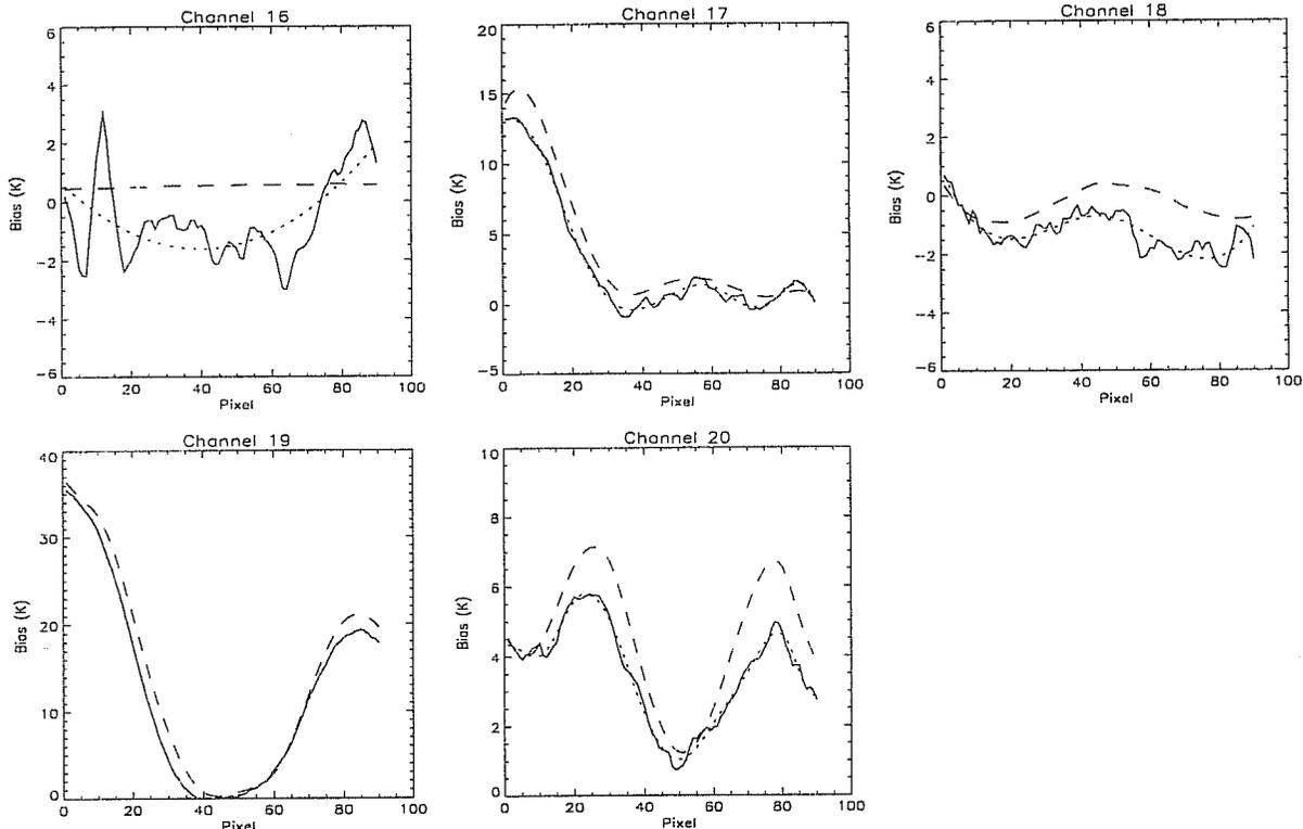
Fig 1: AMSU-B biases (STX-2 omni + SARR) deduced from October 1999 trending test. Solid: raw data from trending test; Dotted: least-squares fit through data; Dashed: Existing AAPP correction tables.
