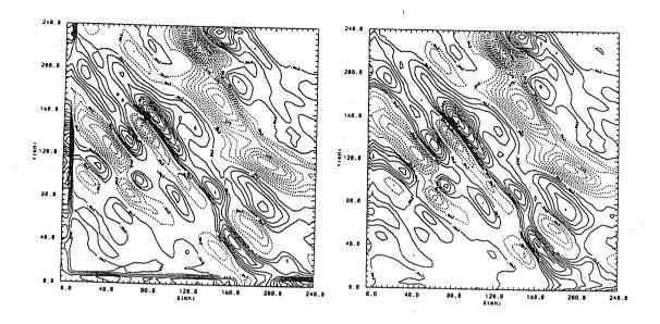
Fig. 5 Plots of w at z=4 km above a surface reference level for flow over the Mogollon rim area of Arizona. (a) shows results using (78) with  $\epsilon=1$  and (b) shows results with  $\epsilon=.025$ .
