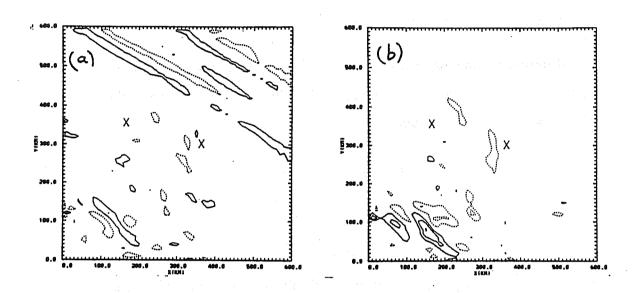
Fig. 4 Plots of vertical vorticity at z=8 km above a ground reference level for flow over the Colorado Rockies. (a) shows results using (77) with  $\epsilon=1.0$  and (b) shows results using  $\epsilon=1$ .
