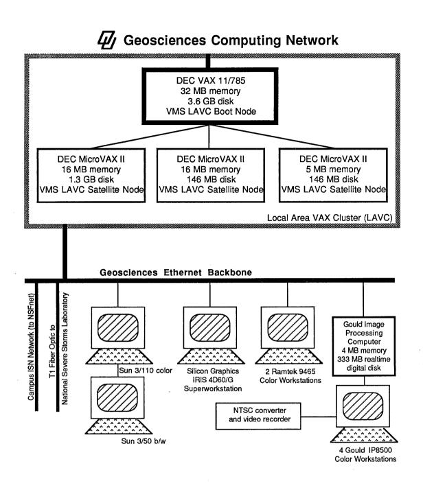
Figure 1. Schematic of the Geosciences Computing Network (GCN) at the College of Geosciences, University of Oklahoma. See the text for further details.
